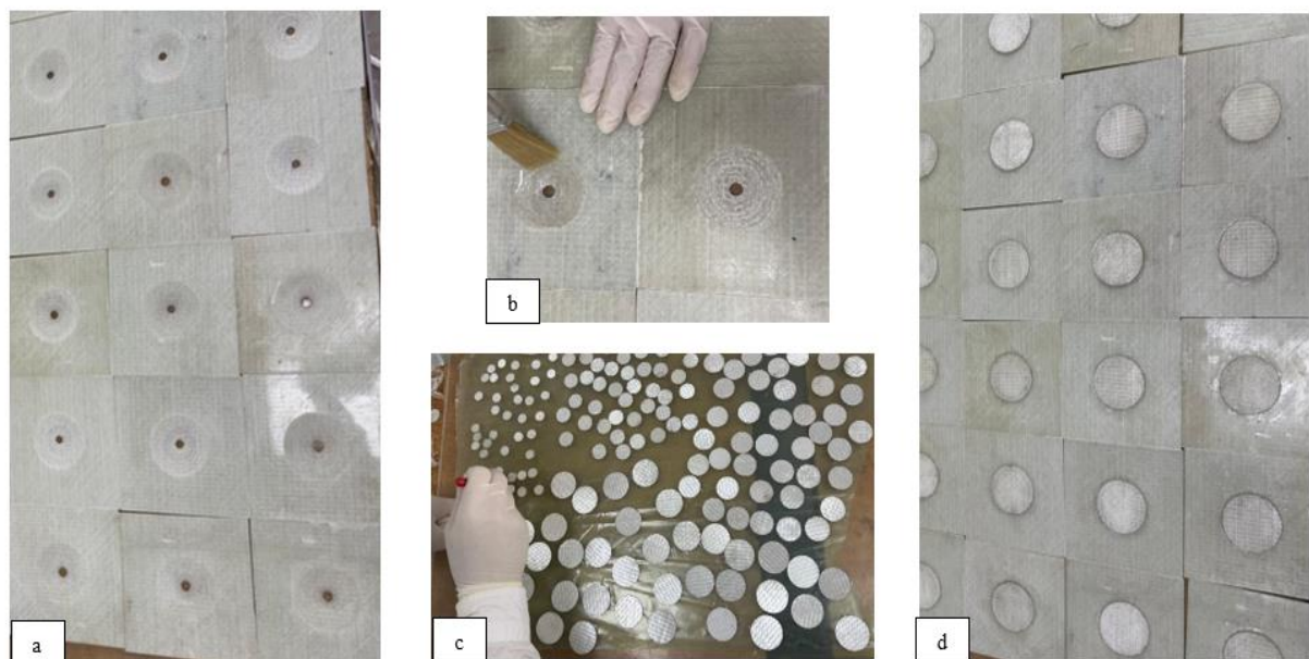
Figure 2. a) specimens after sanding, b) Resin applied, c) plies rolled with resin, d) final specimens before applying biaxial loading
