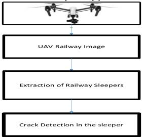
Figure 2. Structure of the described procedure for finding crack faults in sleepers.
