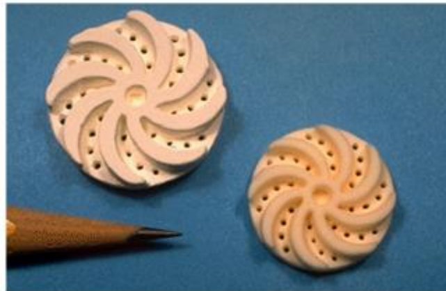
Figure 3. Structural alumina part before (left) and after (right) sintering with shrinkage [36]
