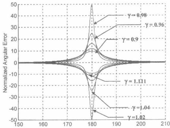
Fig. 3 Normalized Induced Jamming Error vs. Effective Phase Difference
