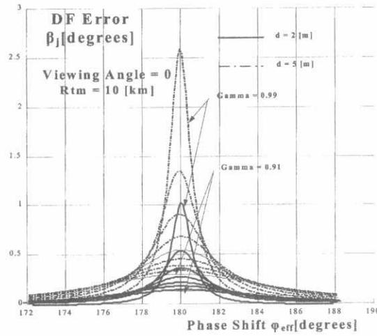
Fig.2 Variation  $\beta_j$  with  $\varphi_{eff}$  and  $\gamma$  at two different values of  $d$
