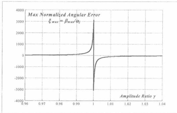
Fig. 4 Maximum value of the normalized induced error vs. the amplitude ratio  $\gamma$
