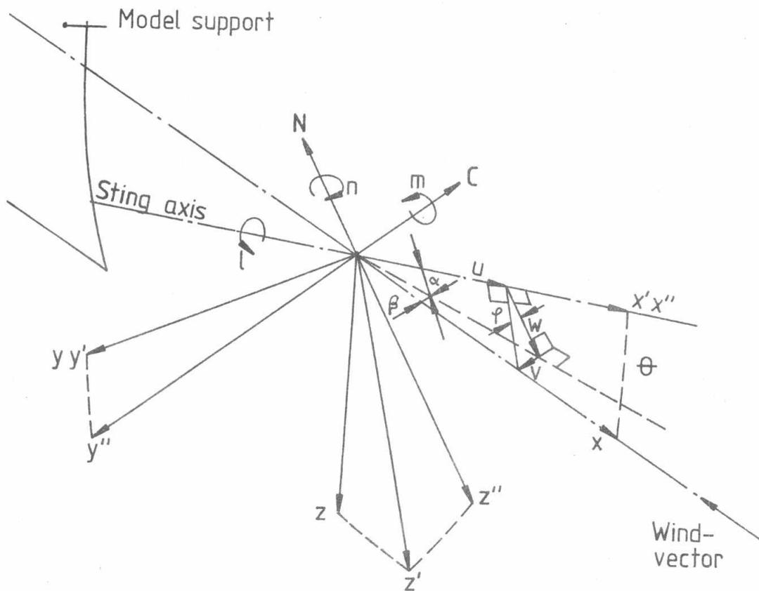
Geometrical relations between aeronautical angles  $\alpha, \beta$  and wind tunnel angles  $\theta, \varphi$
