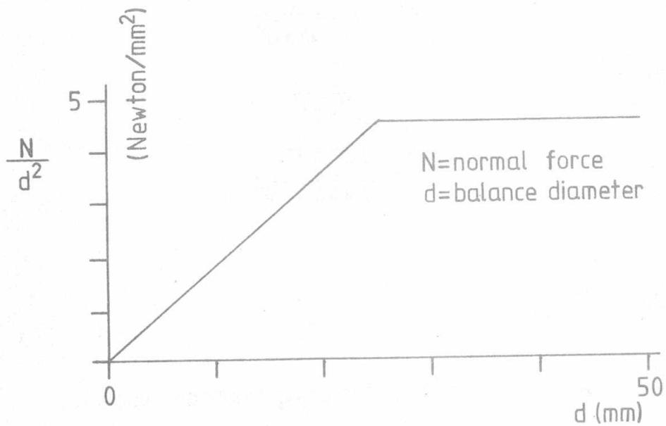
Fig. 13: Approximate limit curve for layout of bending-beam balances.
