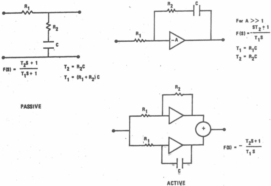
Fig. 2. Filter circuits and their transfer functions.
