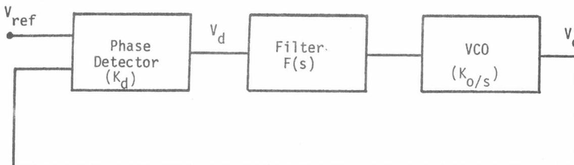
Fig. 1 : Basic phase locking loop
