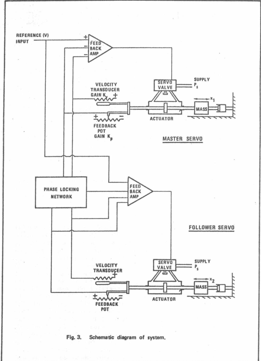
Fig. 3. Schematic diagram of system.
