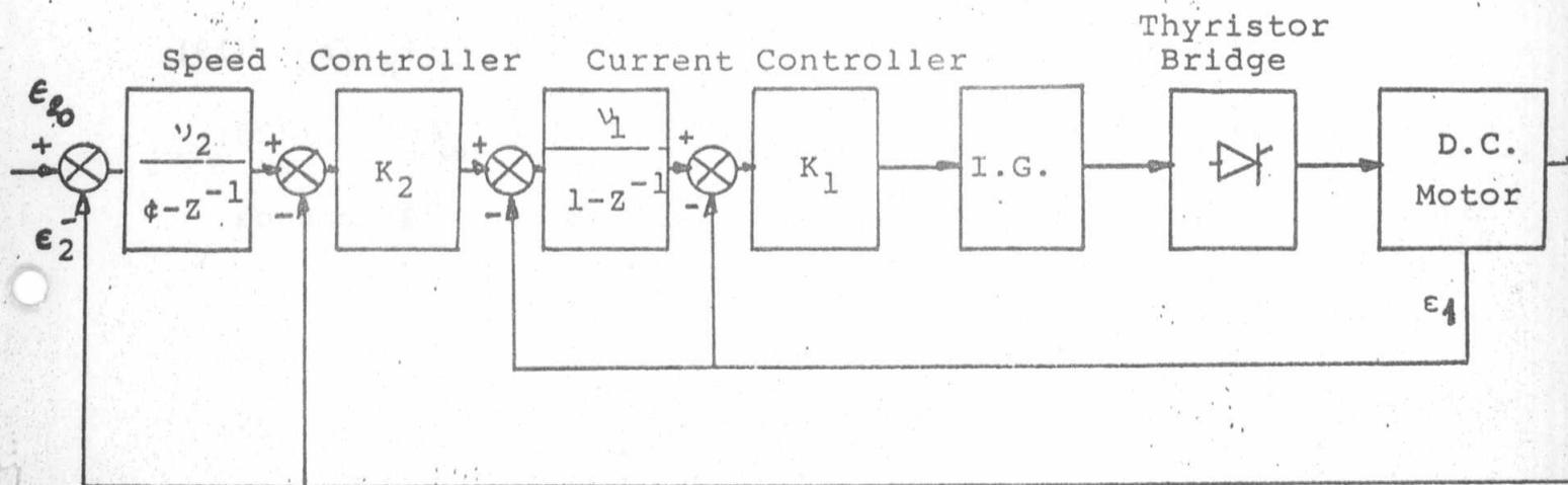
Fig. (3): Block Diagram Using Reduced Variables.
