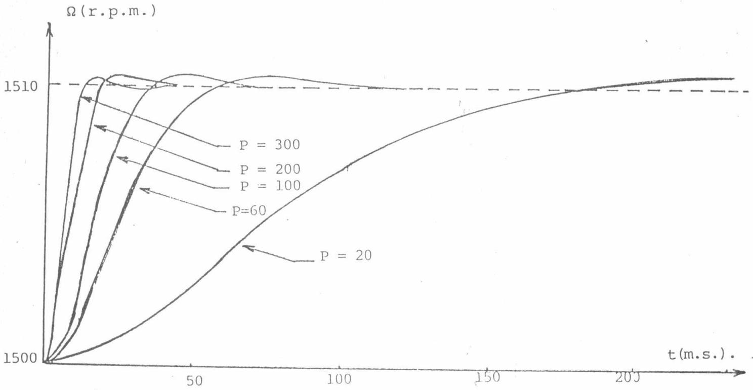
Fig. (4): The System Response Due to Step Change in Speed Reference.
