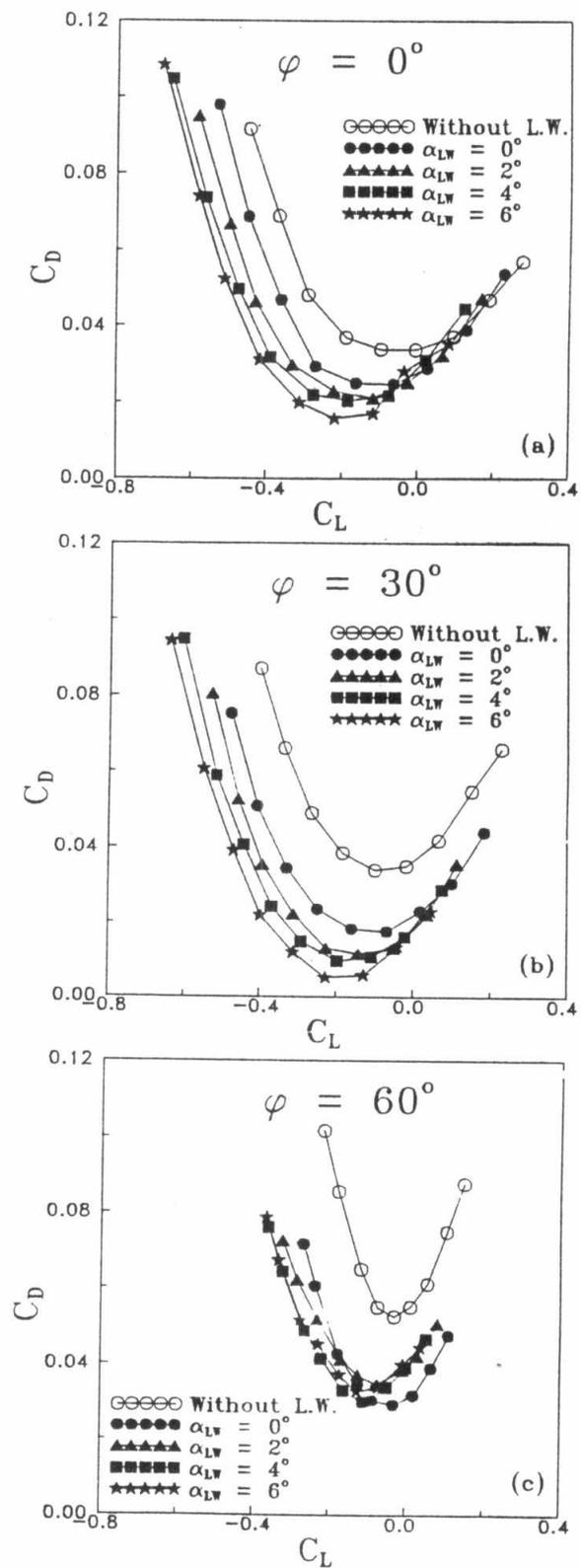
Fig. 5 Drag polar of the trailing configuration for various bank angles and different leading wing settings.
