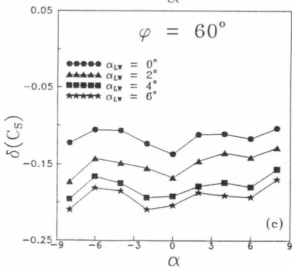
Fig. 10 Change in the yawing moment coefficient caused by trailing vortices.
