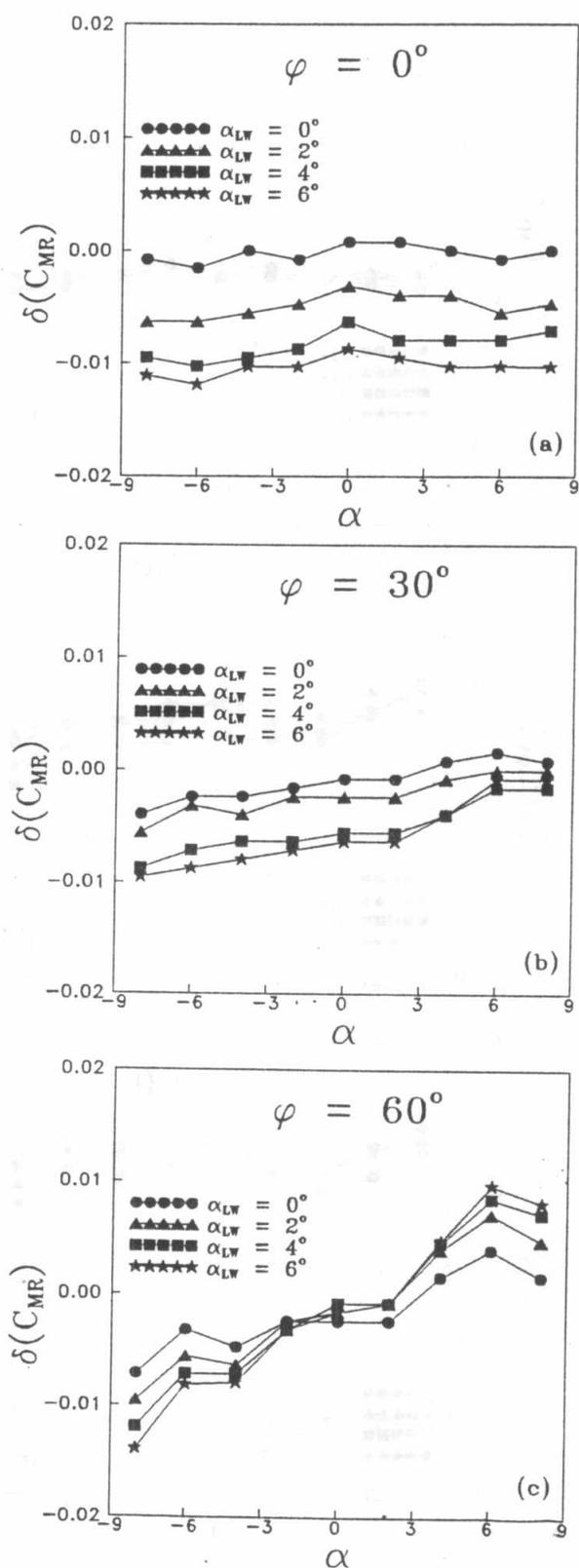
Fig. 9 Change in the rolling moment coefficient caused by trailing vortices.
