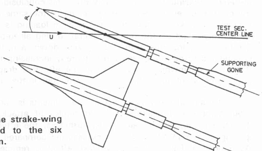
Fig. 1 Schematic of the strake-wing body model connected to the six component balance arm.
