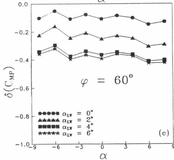
Fig. 6 Pitching moment coefficient for various bank angles and different leading wing settings.
