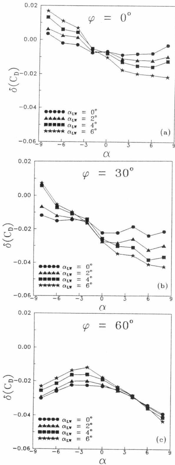
Fig. 4 Change in the drag coefficient caused by trailing vortices for various bank angles.
