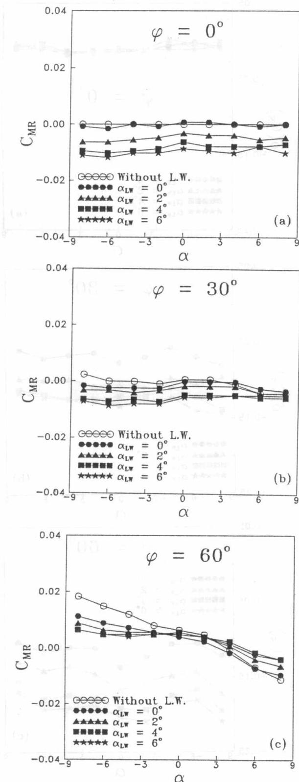
Fig. 8 Rolling moment coefficient for various bank angles and different leading wing settings.
