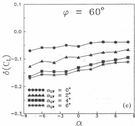
Fig. 2 Lift coefficient of the trailing configuration for various bank angles and different leading wing settings.
