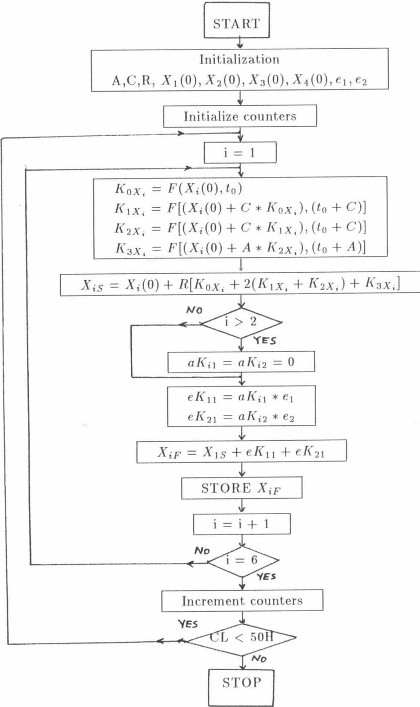
Fig.(5) Flowchart For Calculating State Vector.
