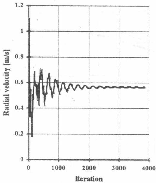
c. Radial velocity component near leading edge.
