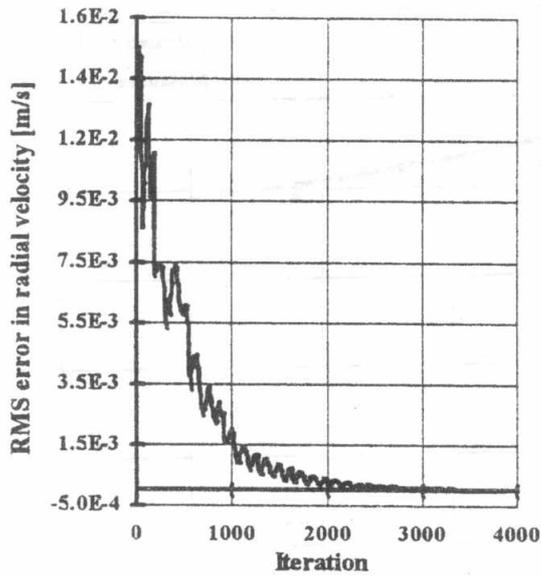
a. RMS error in radial velocity component.
