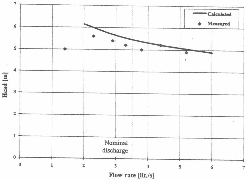
Fig.4 Comparison between the predicted pump performance and the measured values.
