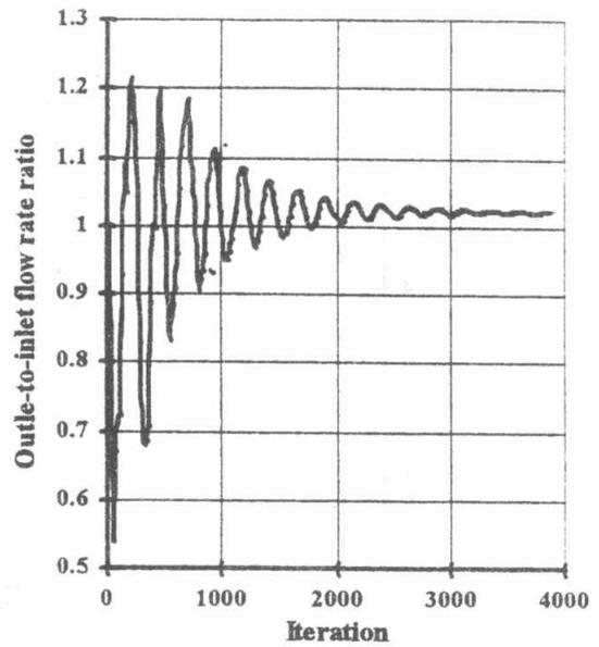
b. Outlet-to-inlet flow rate ratio.
