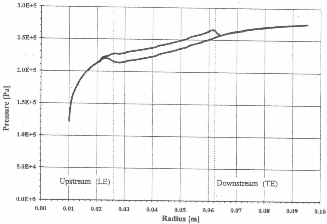
Fig.5 The static pressure distribution on the pressure and suction sides of the impeller.
