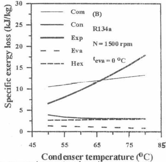
Fig. 4 Effect of condensation temperature on exergy loss rate of each component of the VCHP. A at  $T_{eva}=5^{\circ}\text{C}$  and B at  $T_{eva}=0^{\circ}\text{C}$ .
