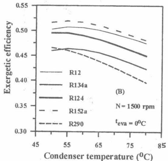
Fig.11 Comparison of useful exergy rate variation for various refrigerants. A at  $T_{eva}=10^\circ\text{C}$  and B at  $t_{eva}=0^\circ\text{C}$ .
