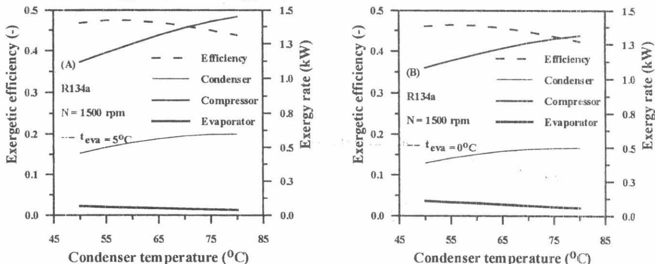
Fig.7 Variation of performance characteristics of the VCHP with the condenser temperature. A at  $T_{eva}=5^{\circ}\text{C}$  and B at  $T_{eva}=0^{\circ}\text{C}$ .
