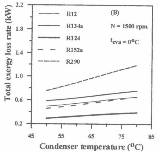
Fig.9 Comparison of total exergy loss rate variation for various refrigerants. A at  $T_{eva}=10^\circ\text{C}$  and B at  $t_{eva}=0^\circ\text{C}$ .
