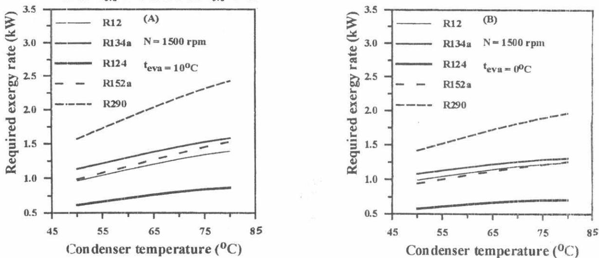
Fig.8 Comparison of required exergy variation for various refrigerants. A at  $T_{eva}=10^{\circ}\text{C}$  and B at  $T_{eva}=0^{\circ}\text{C}$ .
