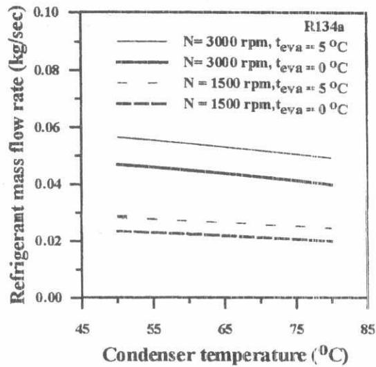
Fig.3 Effect of condensation temperature On refrigerant mass flow rate
