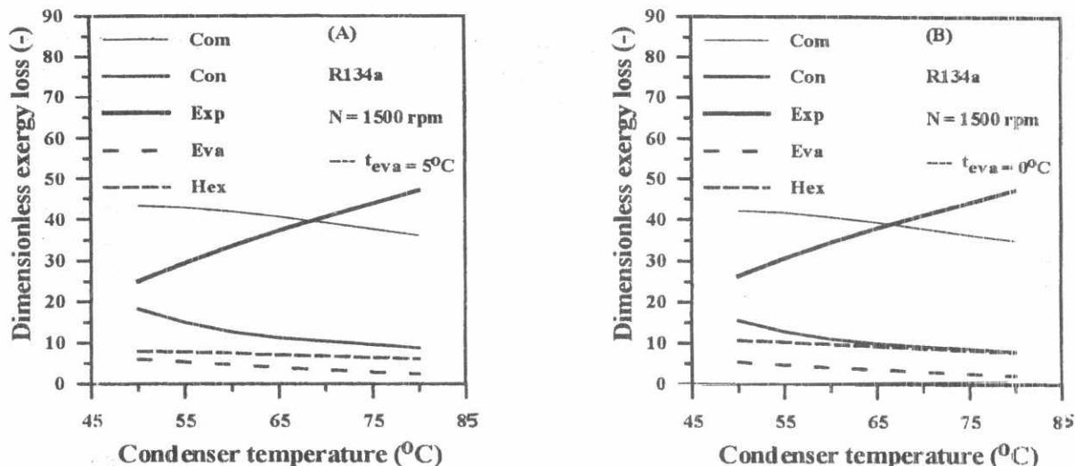
Fig.6 Variation of the dimensionless exergy loss of the main components of the VCHP. A at  $T_{eva}=5^{\circ}\text{C}$  and B at  $T_{eva}=0^{\circ}\text{C}$ .
