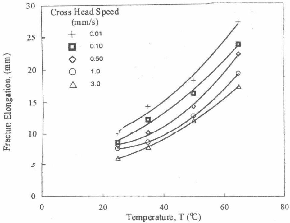
Fig. 5c. Variation of the fracture elongation versus temperature and cross head speed.
