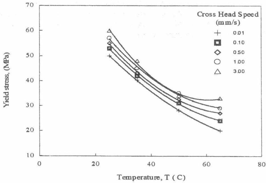
Fig. 5a. Variation of yield stress versus temperature and cross head speed.
