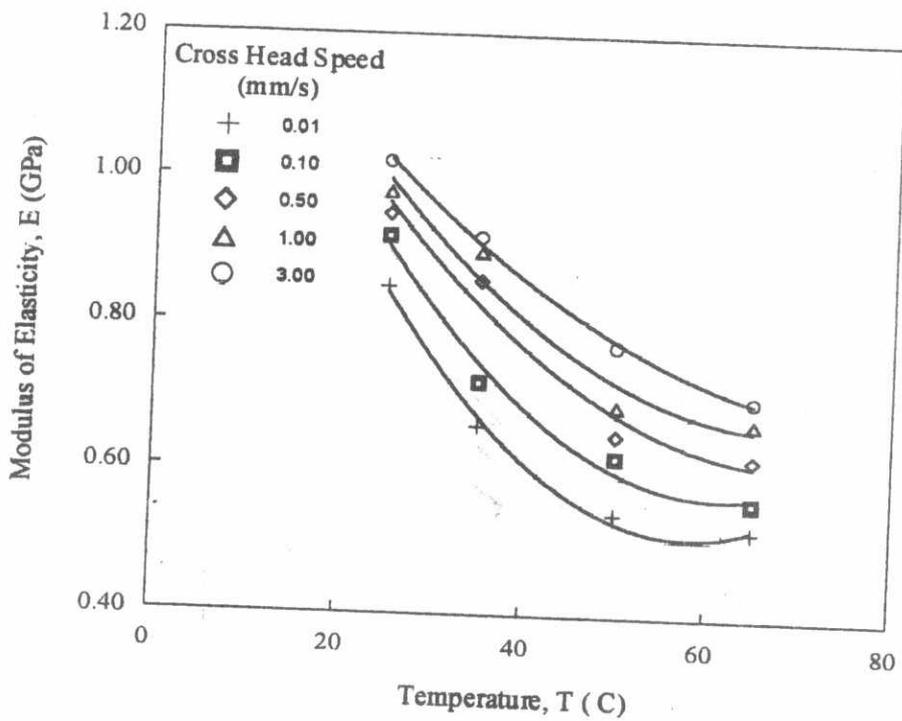
Fig. 5b. Variation of the Modulus of elasticity versus temperature and cross head speed.
