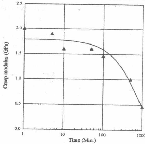
Fig. 10. Variation of the creep modulus with time
