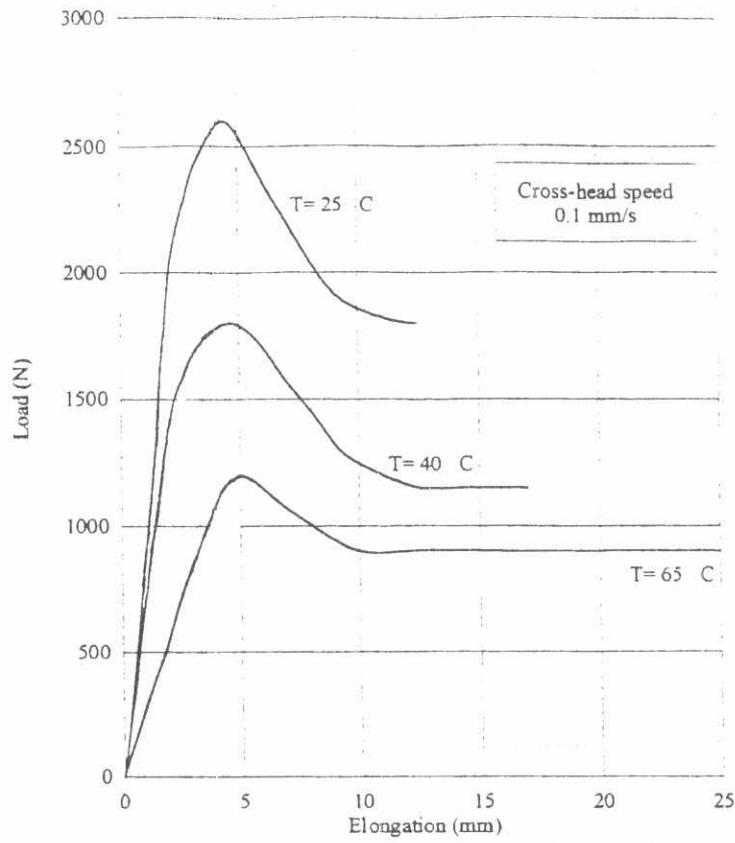
Fig. 3. Load-elongation curves at different temperatures and cross-head speed of 0.1 mm/s.
