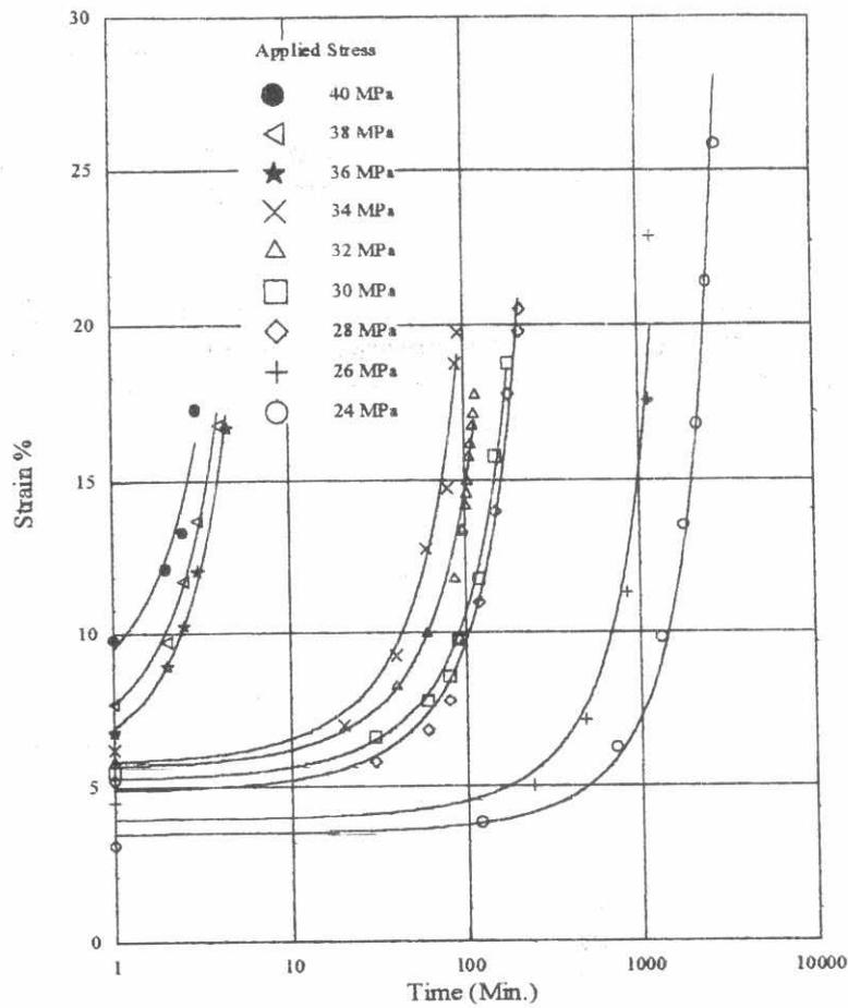
Fig. 7. Creep curves of a PVC specimens subjected to different stress levels
