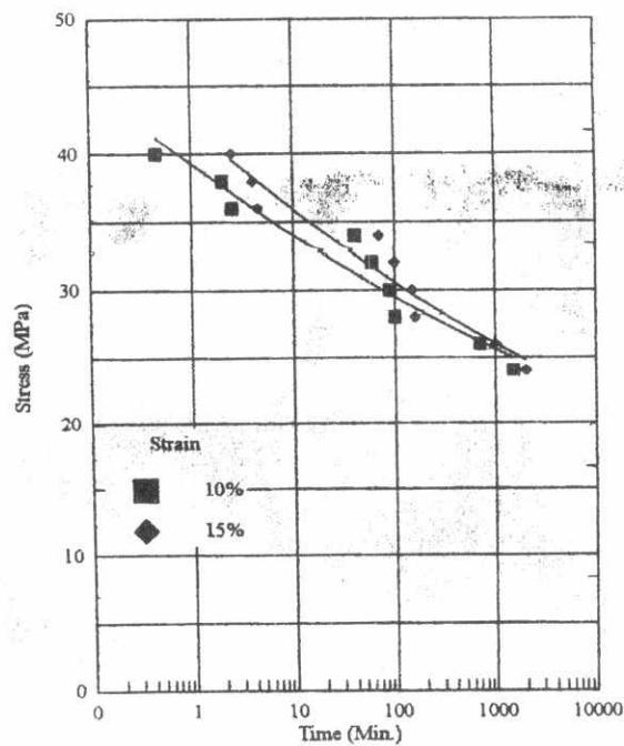
Fig. 8. Stress-Time curves for PVC at 30 °C At two different strain values.
