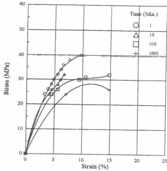
Fig. .9. Isochronance stress-strain curves for PVC at 30 °C at various times.
