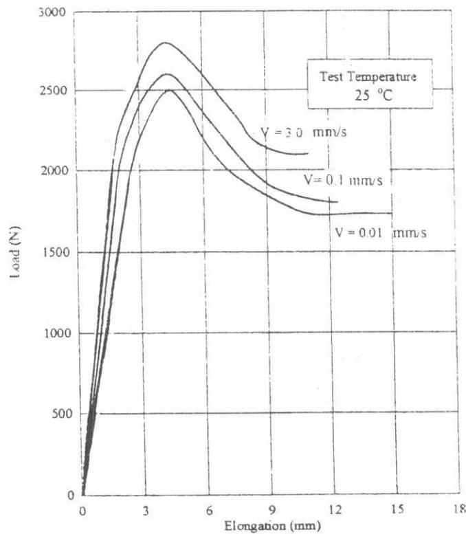
Fig. 4. Load-elongation curves at different cross-head speed and a temperature of 25°C
