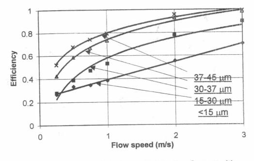
Fig.4 Cyclone Effeciency of Collecting Cement with Different Particle Size
