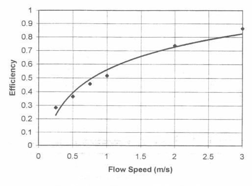
Fig.3 Cyclone Efficiency of Collecting Cement Powder
