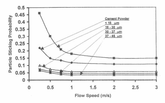
Fig.5 Sticking Probability Versus Flow Speed
