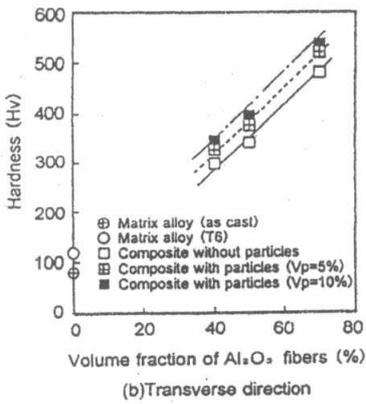
Fig. 7 Effect of volume fraction of fibers and particles on hardness of composites .
