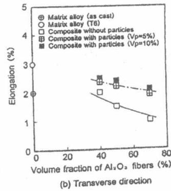
Fig. 6 Effect of volume fraction of fibers and particles on elongation of composites in the longitudinal and transverse directions of the fibers .
