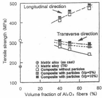
Fig. 5 Effect of volume fraction of fibers and particles on tensile strength of composites.
