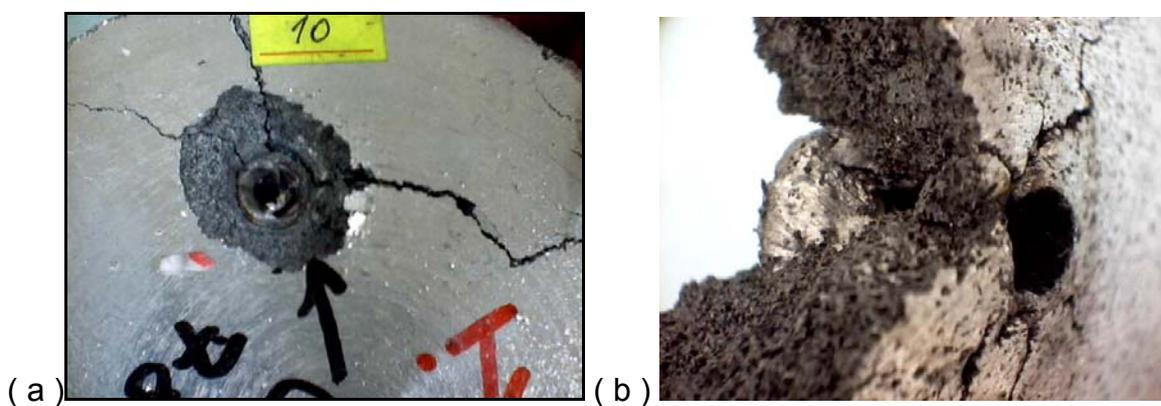
Figure 8. The damage on the Al- 20%SiC Composite target a) entrance of the projectile, b) exit of the projectile
