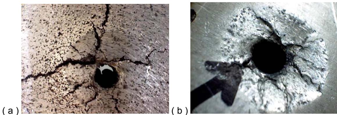
Figure 5. a) Damage on the back surface of the Al- 20%SiC Composite target, b) Damage on the front surface of the Backing Plate
