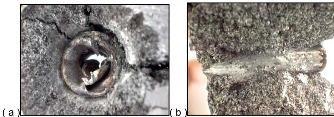
Figure 6. a) The projectile jacket caught by the target, b) The projectile core caught by the target
