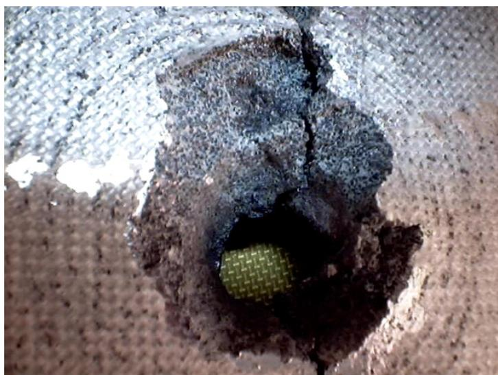
Figure 9. The damage on the Al- 20%SiC Composite target without backing block
