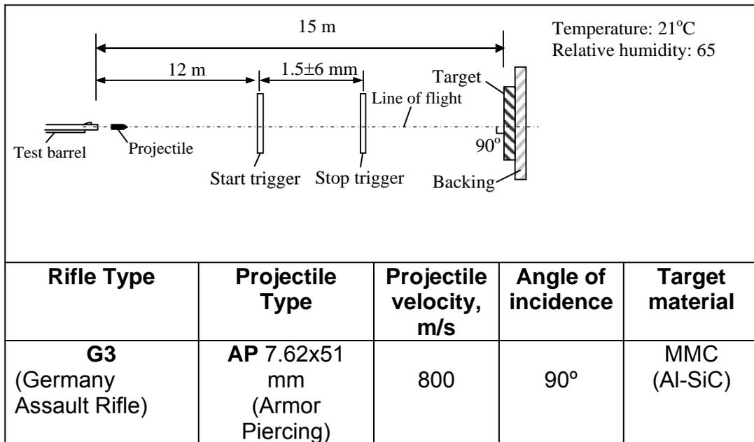
Figure 1. Ballistic test configuration and conditions
