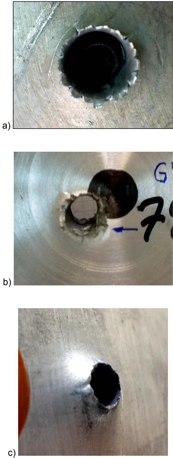
Figure 3. The deformations on the a) front side of the backing plate, b) front side of the unreinforced Al-7075, c) back side of the backing plate used with unreinforced Al-7075
