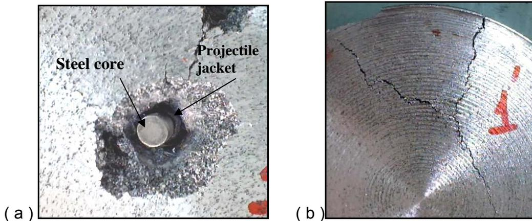
Figure 4. Damages on the Al-20%SiC Composite target a) front surface b) back surface
