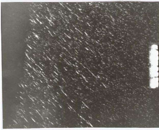
Fig. 11 TEM image in dark field, 160000:1-Tetragonal SIGMA phase Ni<sub>3</sub>Mo, spot (022)
