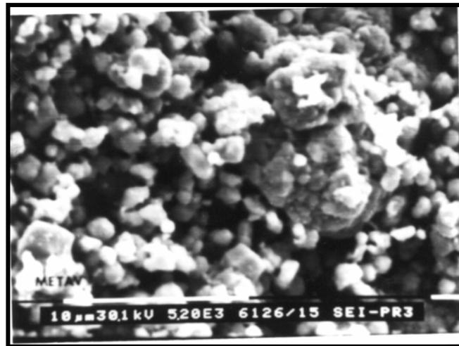
Fig. 4. SEM micrograph of the WNiCu powder mixture after 195 hours ball milling 4780X
