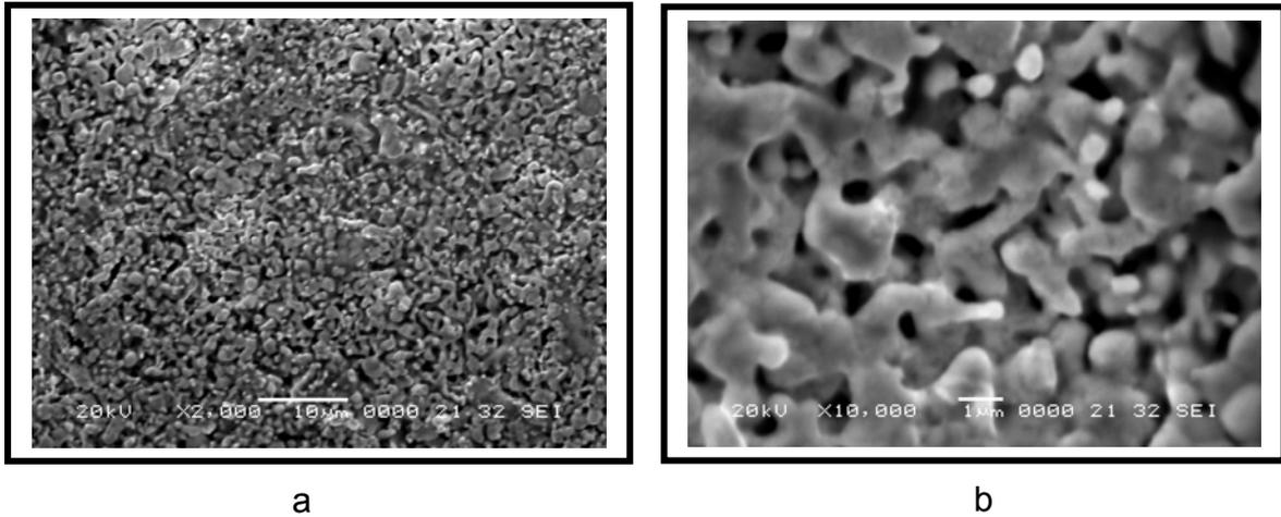
Fig.6. SEM microstructure of the mechanically alloyed  $W_{95}Ni_{3.5}Cu_{1.5}$  powder mixture after sintering for 1 h at  $1250^{\circ}C$
