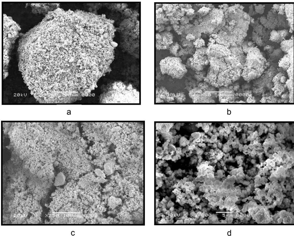
Fig. 5. SEM micrographs revealing the morphological changes of the composite WNiCu powder mixture during the mechanical alloying process
