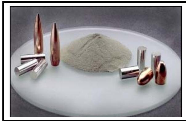
Fig.7. Raw powders – Final products sintered from the mechanically alloyed  $W_{95}Ni_{3.5}Cu_{1.5}$  powder mixture
