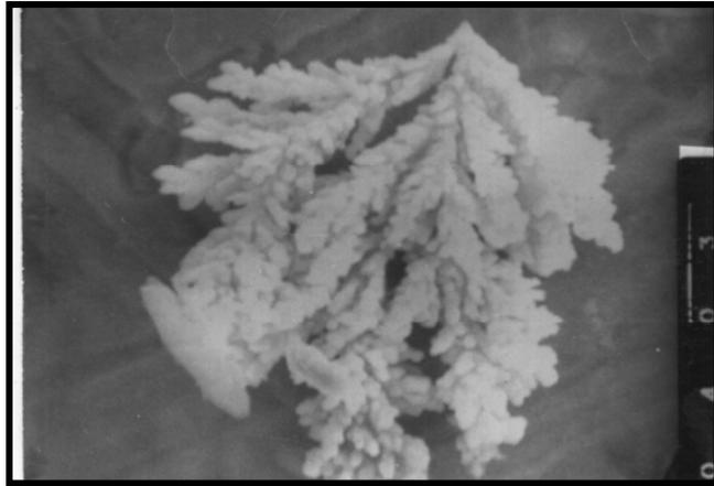
Fig.1. Morphologic aspect of reduced copper powder-particles of dendritic shapes
