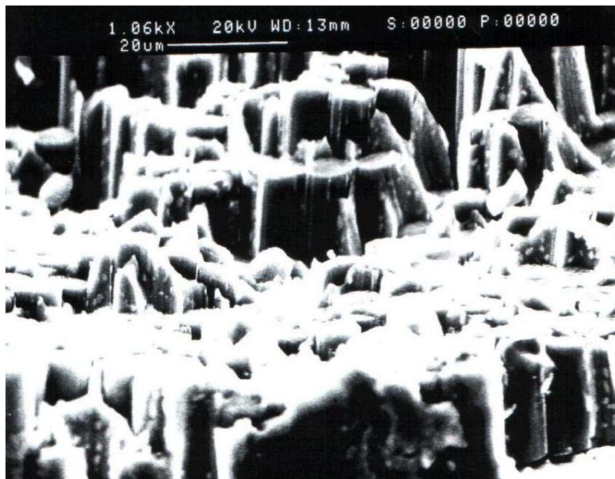
Fig.4. SEM microscopy of a composite with aluminum matrix alloyed with 50% zinc. The length of the extracted fibers can be evaluated by using the ruler above the image
