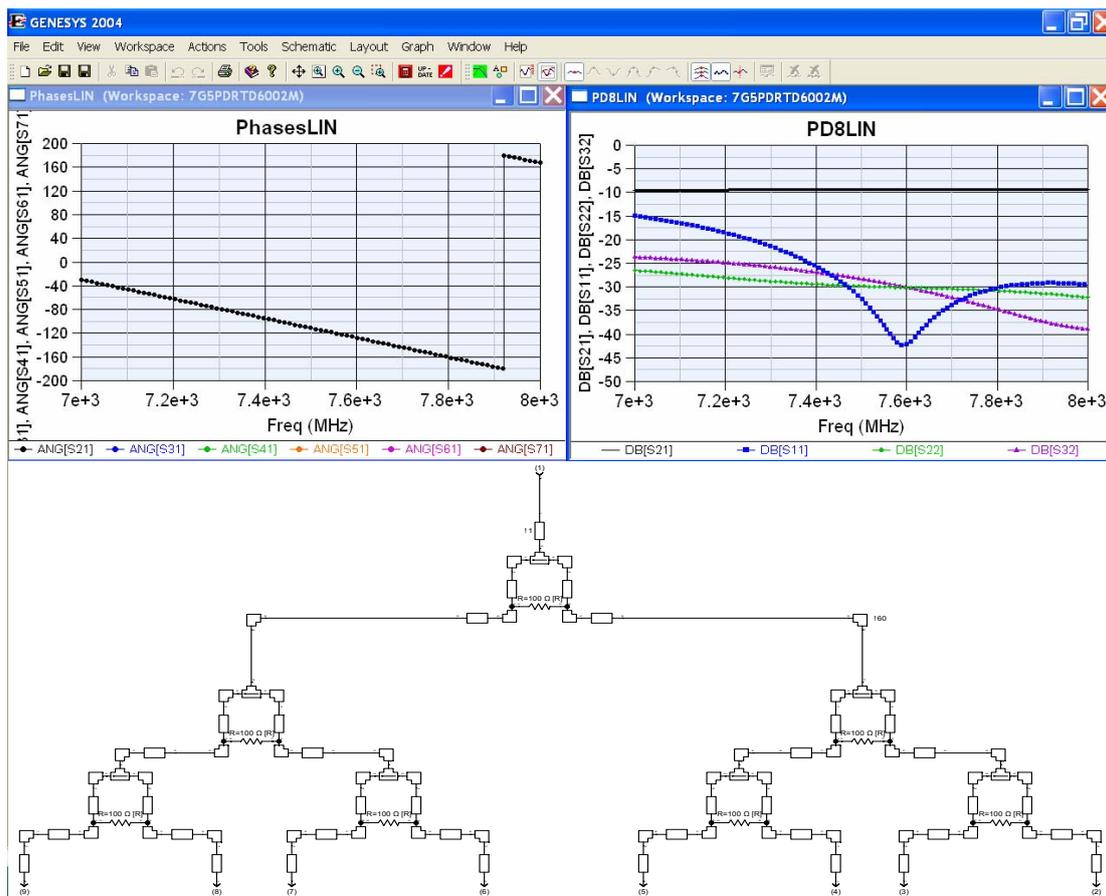
Fig.5. First Run Optimized Linear Simulation
