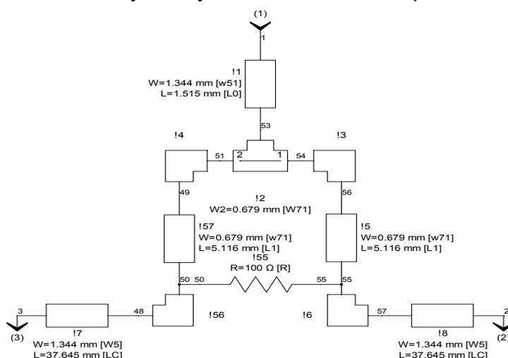
**Fig.1. A two-way Power Divider**
