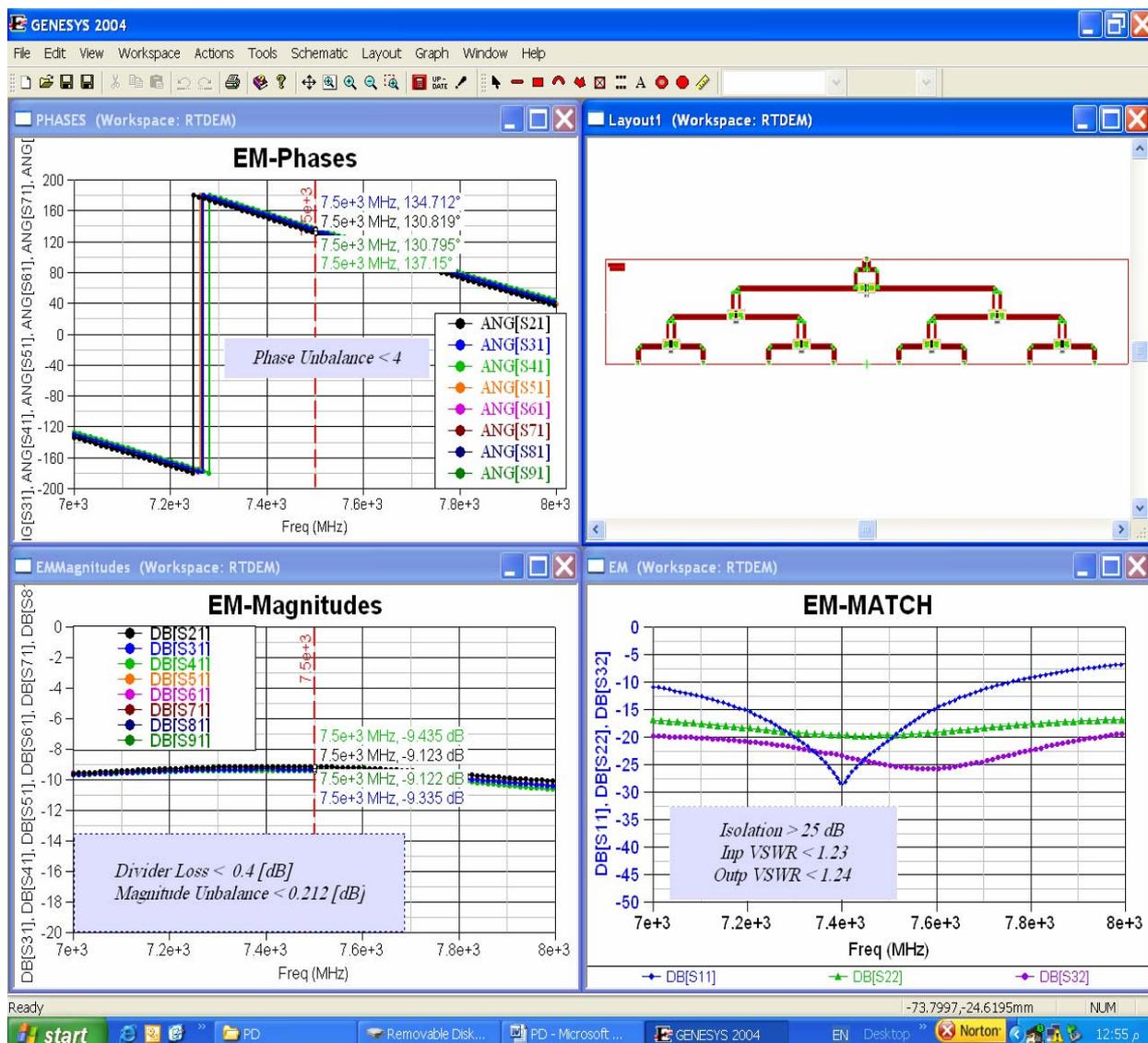
**Fig.9. Layout and Combined simulation results after optimization**
