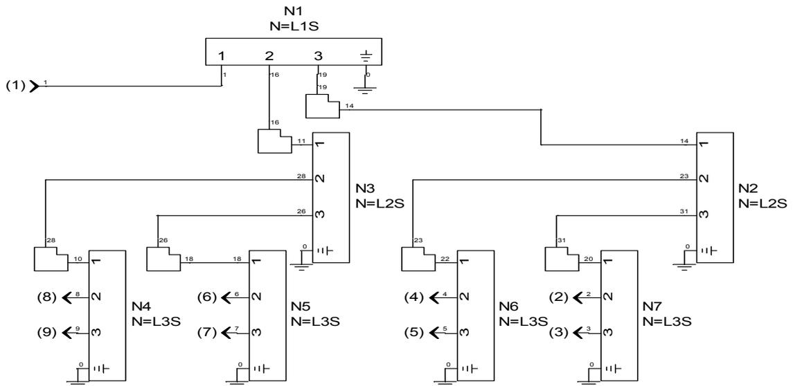
**Fig.3. Cascading 2-way power dividers to construct an 8-way power divider**
