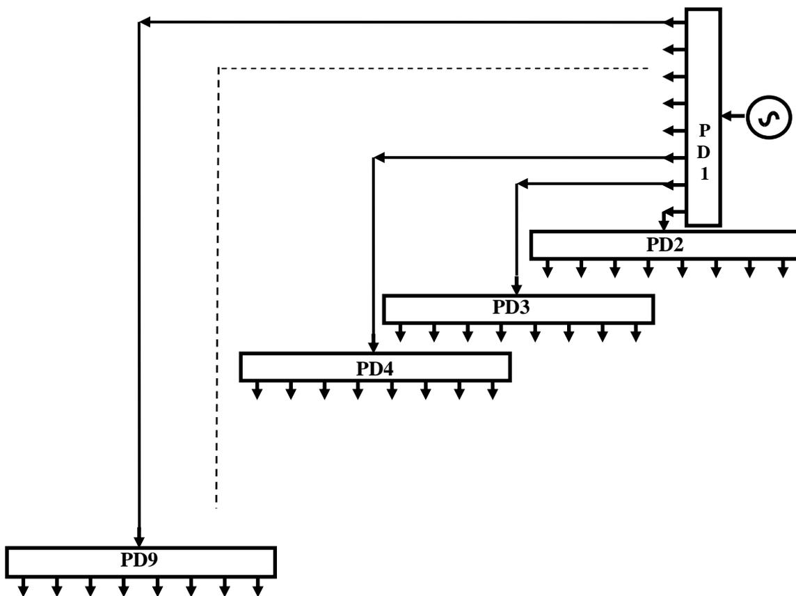
**Fig.11. Local Oscillator Distribution System for an 8x8 array**
