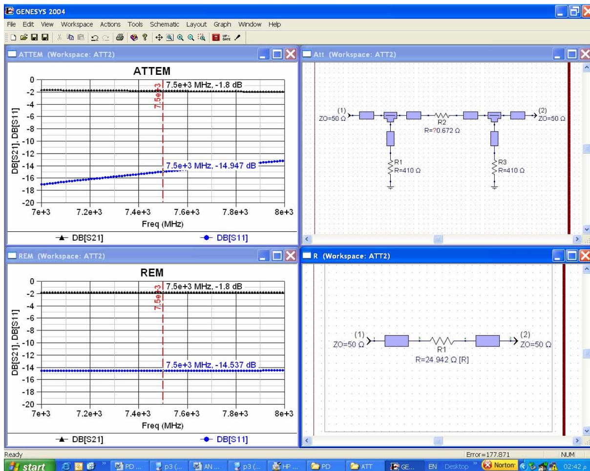
**Fig.10a. A comparison between a PI and a single resistor attenuators**
