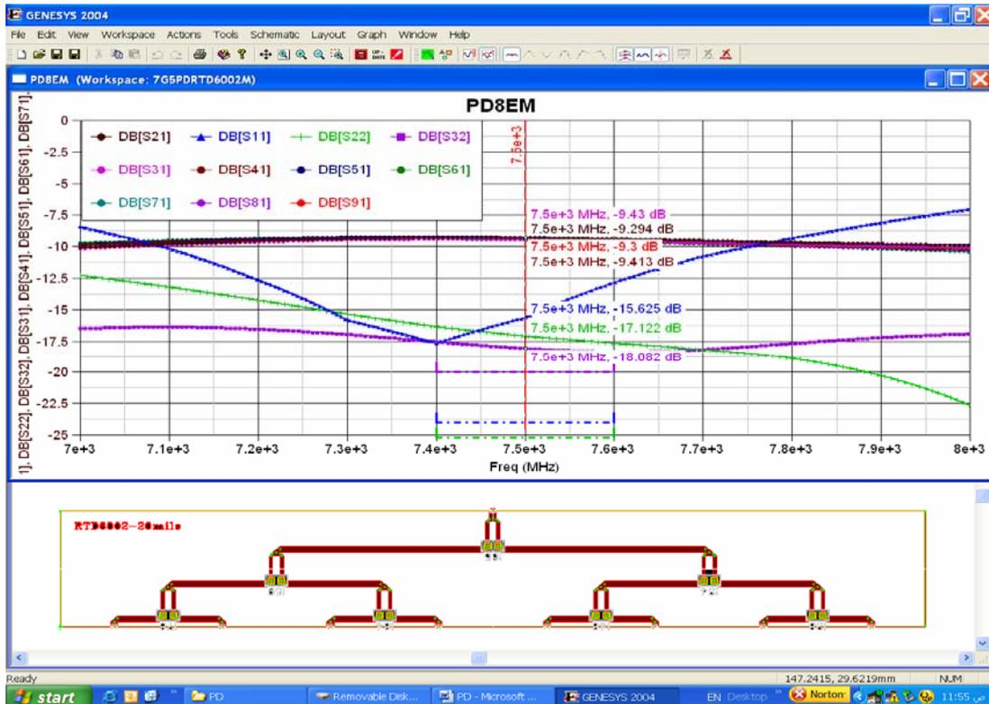
**Fig.6. Layout and EM simulation**
