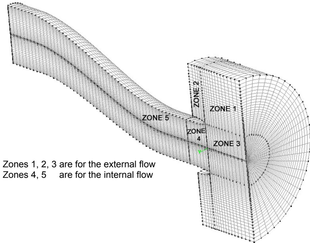
Fig.7. Intake volume grid with the multi zone illustrated
