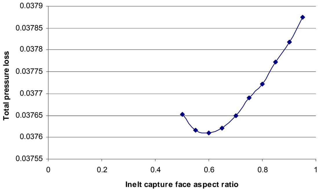
Fig.9. Inlet capture face aspect ratio effect on the total pressure loss
