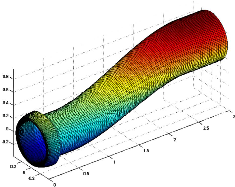
Fig.5. Optimal Intake surface obtained from low fidelity optimization
