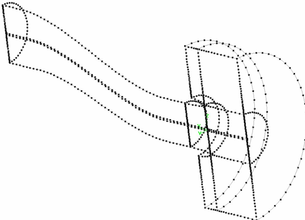
Fig.6. Intake edge grid and clustering
