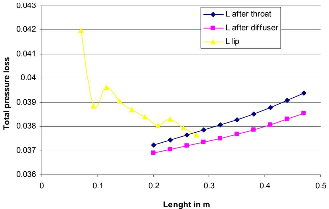
Fig.8. Total pressure losses for lengths variables
