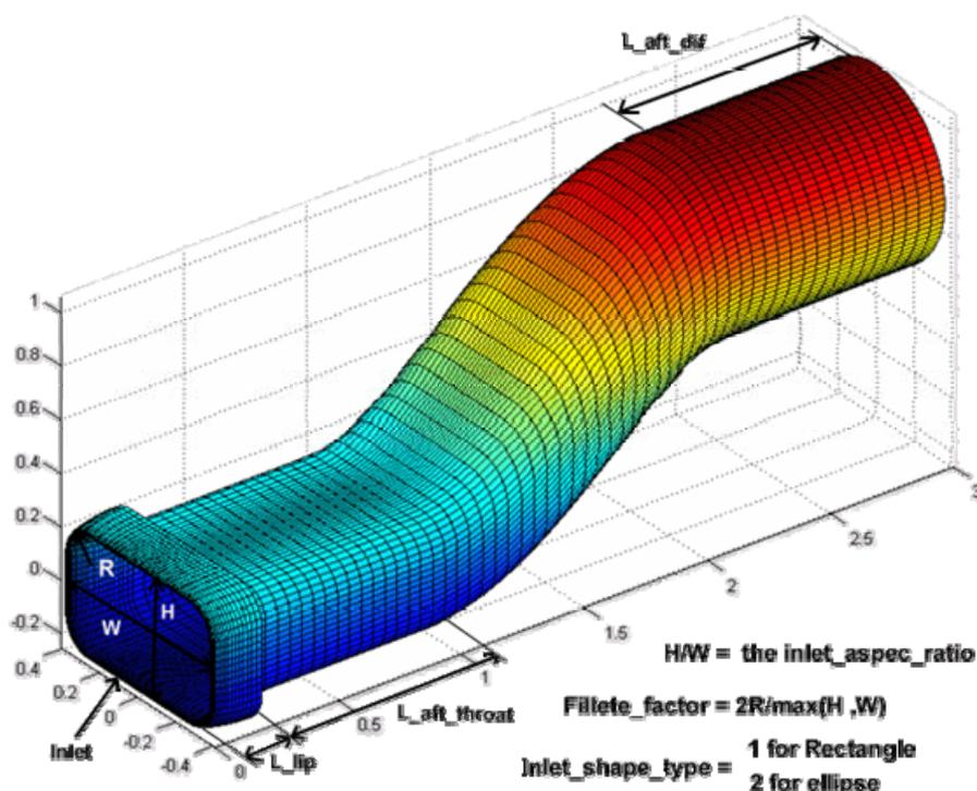
Fig.1. Intake variables illustration
