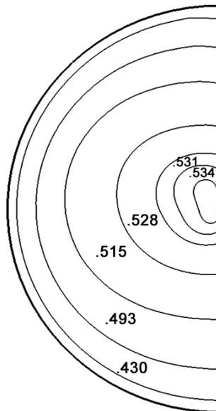
Fig.12. Mach number contours plot for the exit section for the optimal intake
