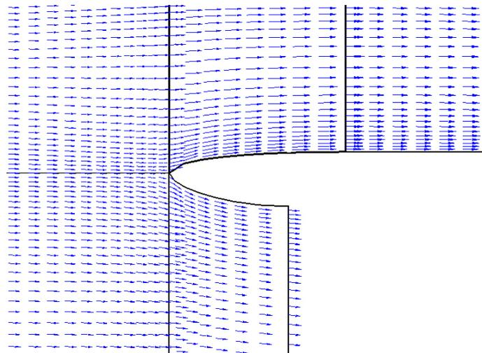
Fig.13. Velocity magnitude and direction vector plot around the lip of the optimal intake
