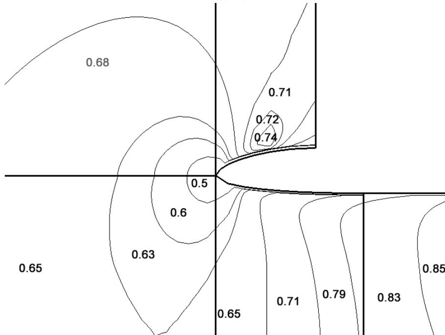
Fig.14 Mach number contours around the lip of the optimal intake
