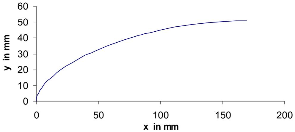
Fig.2. NACA 1 profile for the outer lip
