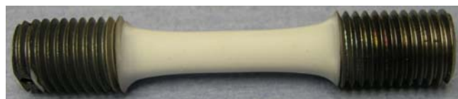
Fig. 2. A TBC coated LCF specimen
