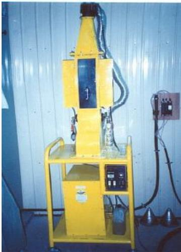
Fig. 3 The smoke tunnel
