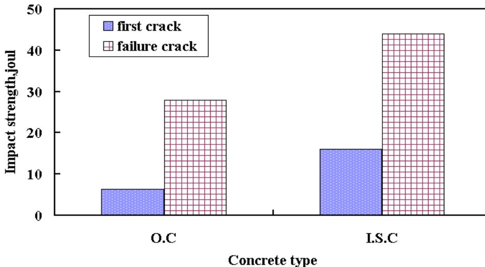
Fig (8) Impact strength of O.C. and I.S.C
