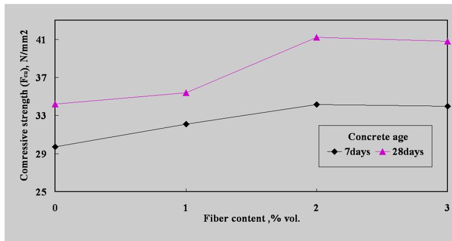
Fig. (5) Compressive strength of I.S.C with different percentages of steel fibers
