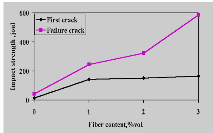
**Fig (9) Impact strength of I.S.F.H.W.C with different percentages of steel fibers**
