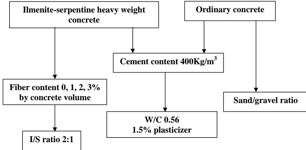
Fig.(2) Scheme of Different Concrete Mixes of Ilmenite-Serpentine Heavy Weight Concrete and Ordinary Concrete.
