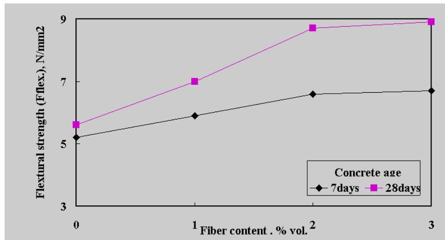
Fig. (7) Flexural strength of I.S.C with different percentages of steel fibers
