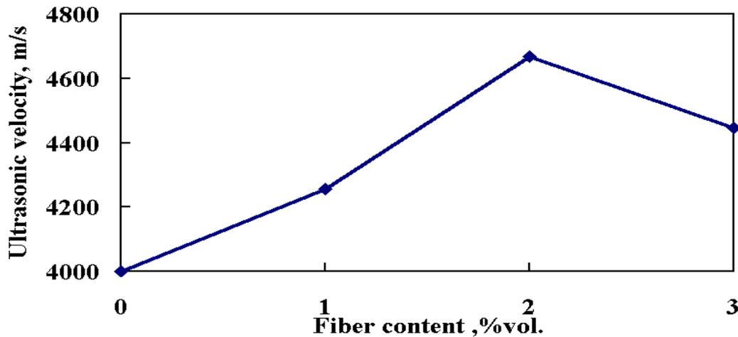
Fig. (4) Ultrasonic velocity values of I.S.C. with different percentages of steel fiber
