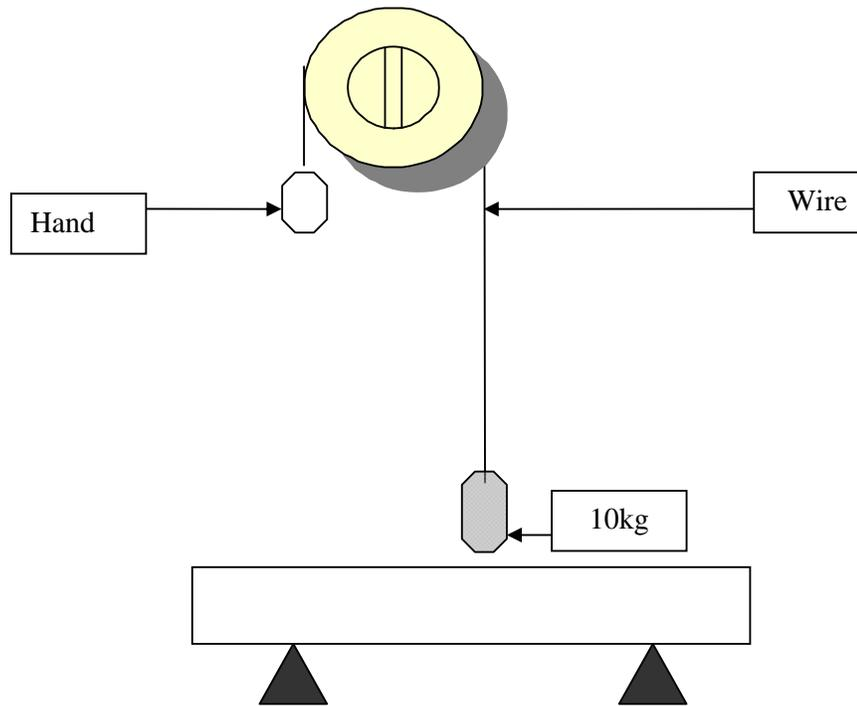
**Fig.(3) The Falling Weight Method**
