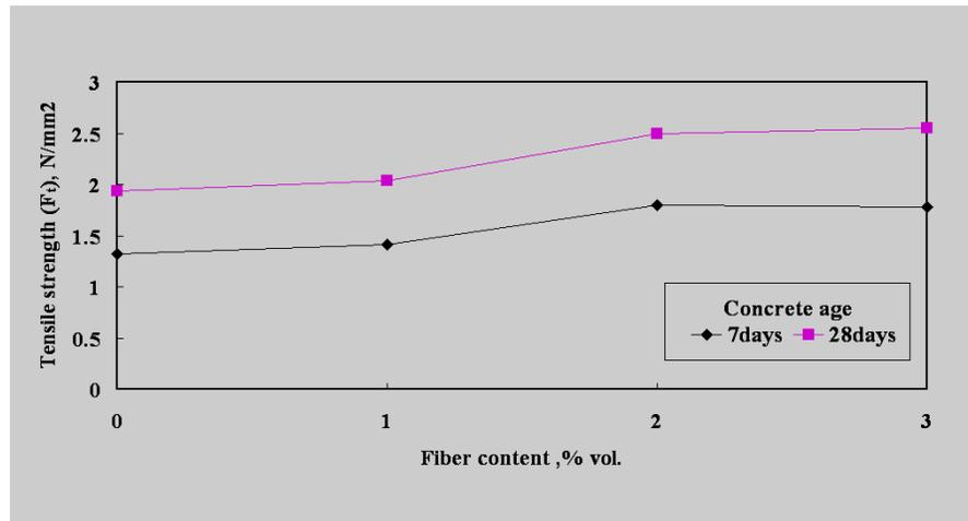
Fig. (6) Tensile strength of I.S.C with different percentages of steel fibers
