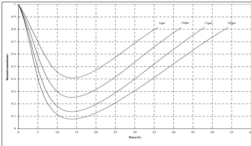
**Figure (3.2) Attenuation of infrared radiation emitted from black body radiator at 100°C by silica foam at relative humidity 35% and ambient temperature 18°C.**
