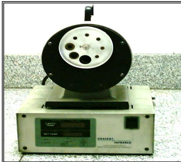
**Figure (2.4) Graseby infrared black body IR radiator with temperature controlling.**
