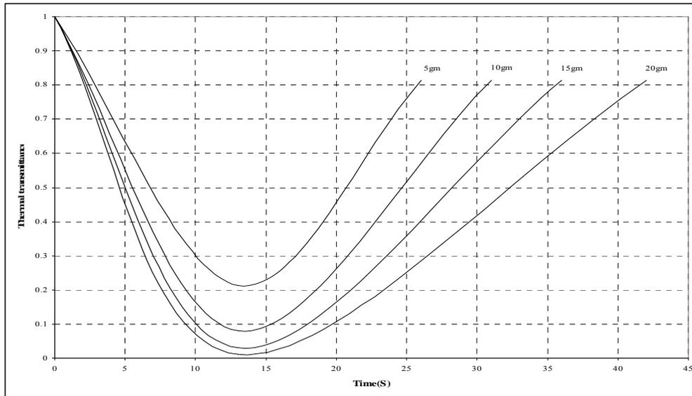
**Figure (3.3) Attenuation of infrared radiation emitted from infrared black body radiator at 100°C by cement-dust at relative humidity 35% and ambient temperature 18°C.**
