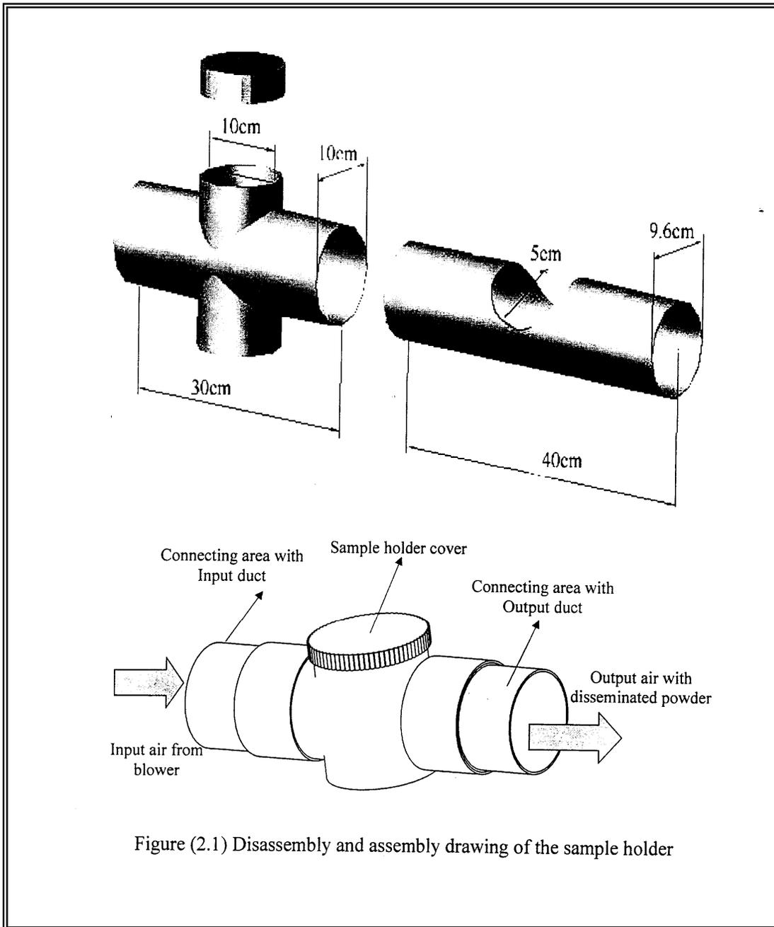
Figure (2.1) Disassembly and assembly drawing of the sample holder
