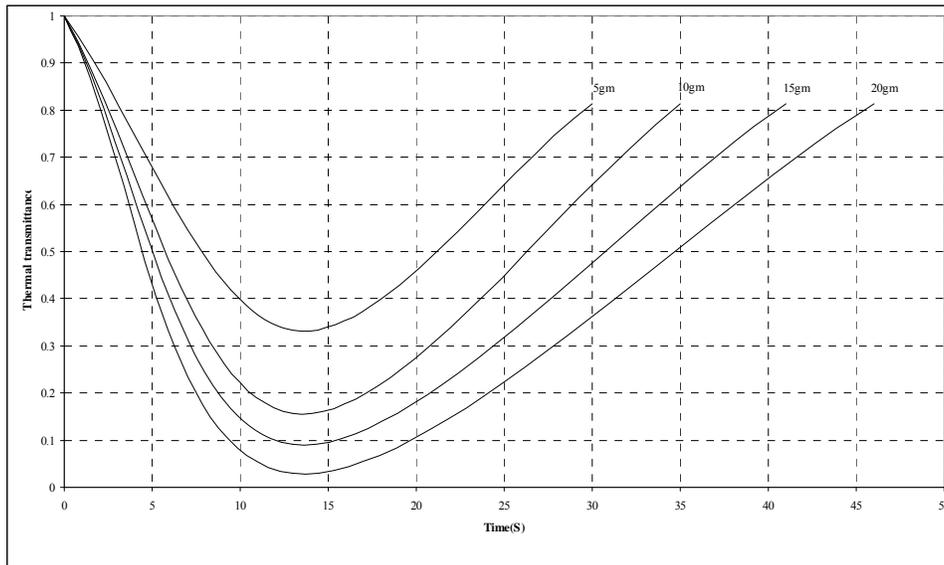
**Figure (3.1) Attenuation of infrared radiation emitted from black body radiator at 100°C by fly ash at relative humidity 35% and ambient temperature 18°C**
