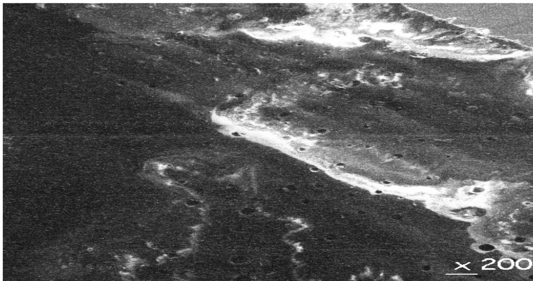
**Fig. 5a** SEM micrograph of 10 phr HTPB blends showing stress-whitened zone.
