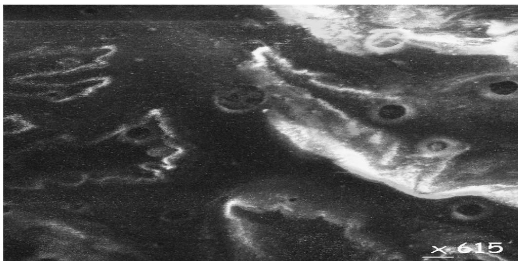
**Fig. 5d** SEM micrograph for 15- phr rubber-modified epoxies.
