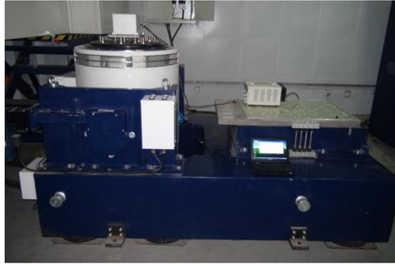
Fig. 9: Vibration shaker test bench
