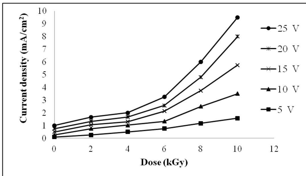
**Fig. 3.** Dependence of the current density with gamma radiation dose for AN-free aluminium oxide film
