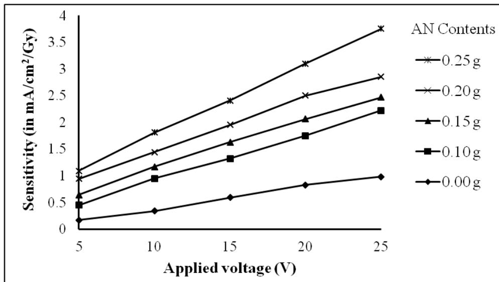
**Fig. 13.** Sensitivity for gamma radiation for different films of different AN content
