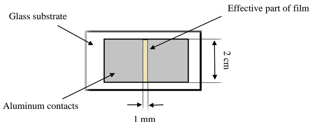
**Fig. 1.** Coplanar structure of a film for the current-voltage measurements
