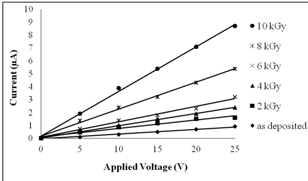
**Fig. 5.** Typical current-voltage characteristics for Aluminium oxide film doped with 0.1gAN exposed to different levels of the gamma radiation dose.
