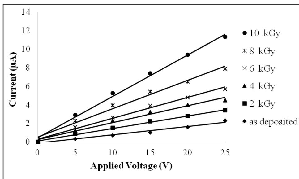
**Fig. 6.** Typical current-voltage characteristics for Aluminium oxide film doped with 0.15g exposed to different levels of the gamma radiation dose
