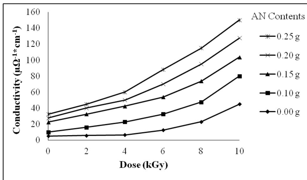
**Fig. 14.** Conductivity for different films at different AN content due to gamma radiation
