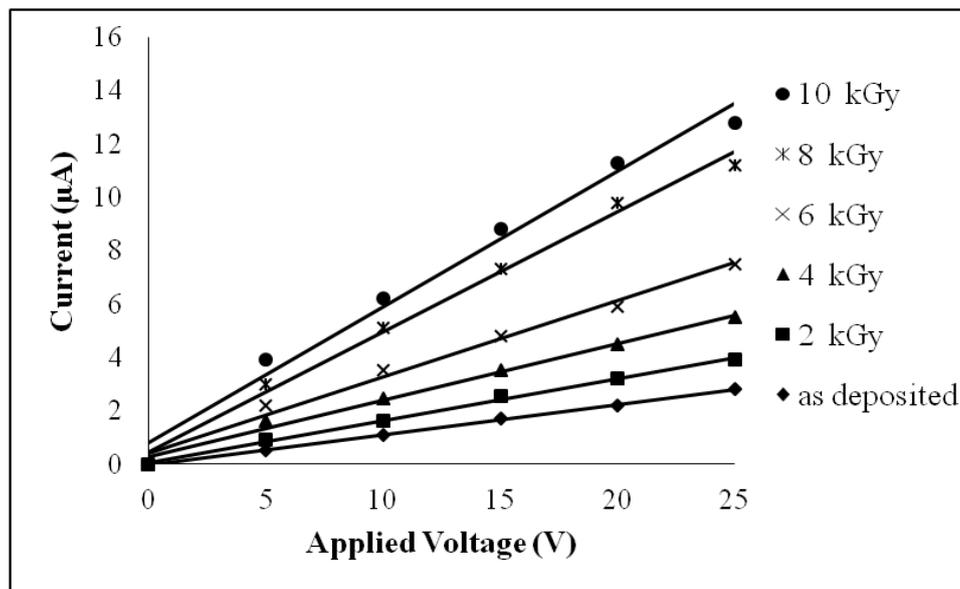
**Fig. 7.** Typical current-voltage characteristics for Aluminium oxide film doped with 0.2g AN exposed to different levels of the gamma radiation dose**Table 5.** The fitted linear equations represent the relation between induced current and applied volt for Aluminium oxide film doped with 0.2 g AN
