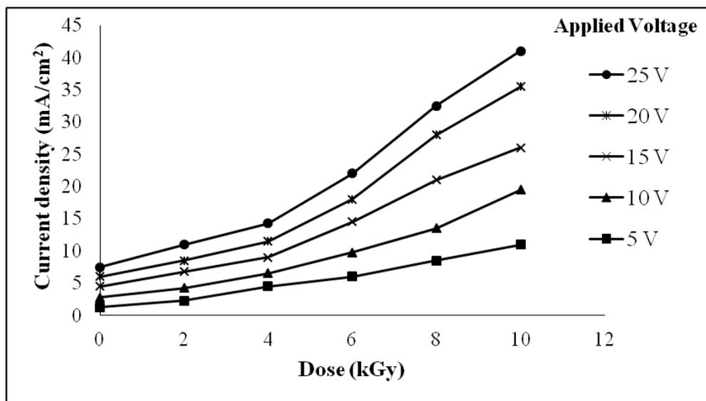
**Fig. 12.** Variation of the current density with gamma radiation dose for aluminium oxide film doped with 0.25g AN
