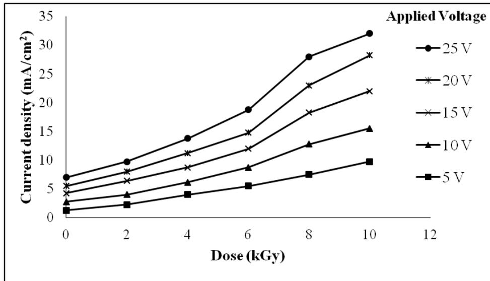
**Fig. 11.** Variation of the current density with gamma radiation dose for aluminium oxide film doped with 0.2g AN
