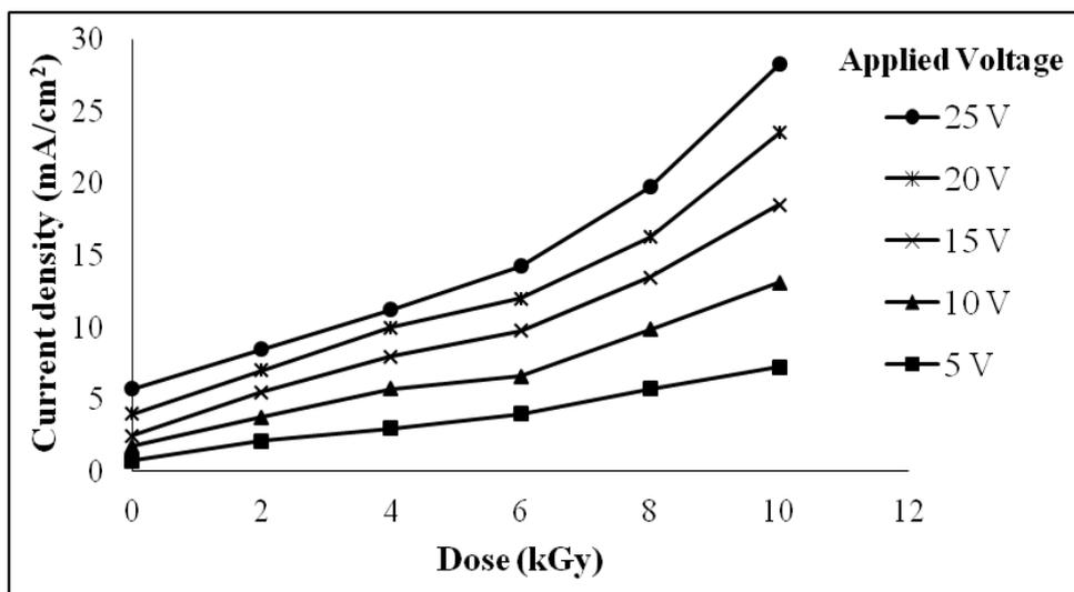
**Fig. 10.** Variation of the current density with gamma radiation dose for aluminium oxide film doped with 0.15g AN
