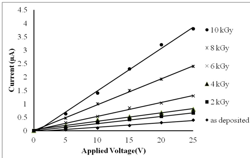
**Fig. 2.** Typical current-voltage characteristics for Aluminium oxide film free from AN exposed to different levels of the gamma radiation dose.
