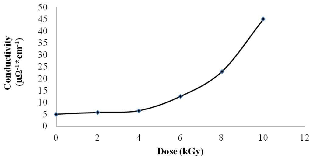
**Fig. 4.** Dependence of conductivity with gamma radiation dose for AN-free aluminium oxide film
