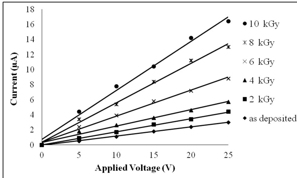
**Fig. 8.** Typical current-voltage characteristics for Aluminium oxide film doped with (0.25g AN) exposed to different levels of the gamma radiation dose.
