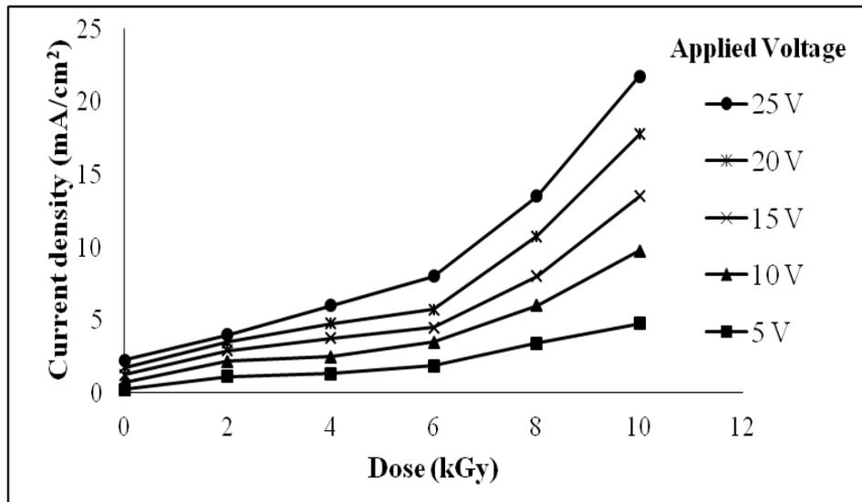
**Fig. 9.** Variation of the current density with gamma radiation dose for aluminium oxide film doped with 0.1g AN
