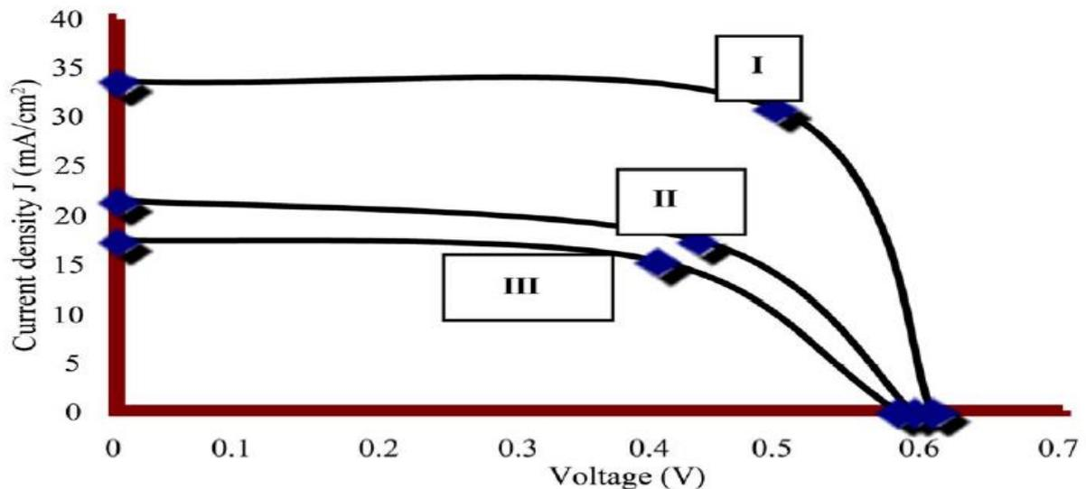
**Fig. 5: Typical I-V Characteristics of an illuminated single crystal silicon solar cell at different values of solar radiation  $100 \text{ mW}/\text{cm}^2$ ,  $60 \text{ mW}/\text{cm}^2$  and  $40 \text{ mW}/\text{cm}^2$  respectively. The open voltage potential is affected only by the temperature of the source of radiation, the sun, while the intensity of solar adiation influences the current density.**
