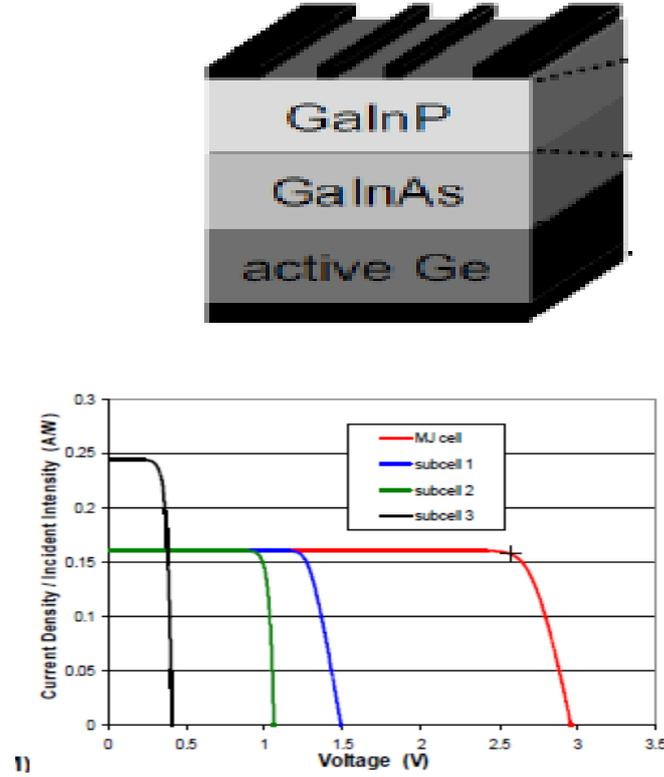
**Fig. 6: Simple cross-sectional diagram and modeled IV characteristics of a typical triple junction solar cell GaInP/GaInAs/ Ge stacked on top of each other. The IV characteristics of each subcell and the whole multijunction solar cell, in red color, are seen under 1x concentration [25]**
