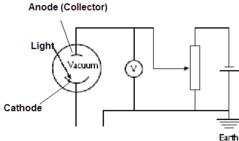
**Fig. 3:** The photocell experiment is designed to measure the stopping potential on the anode (collector) that stops the flow of electric current from the cathode by applying a negative potential on the anode. The incident light is reflected on a Silicon cathode plate with an electric potential that is proportional to the difference between temperature of the source of radiation and the cathode plate..
