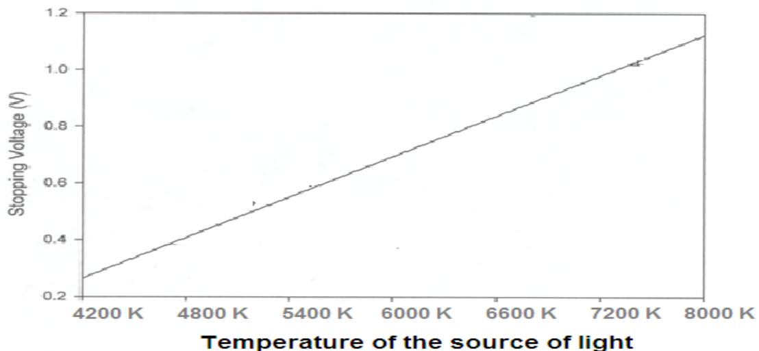
**Fig. 4:** Dependence of the stopping voltage in a photoelectric cell on the temperature of the source of light. The found slope for Sodium plate, as found in the current measurement, is identical to the measured slope for potassium plate as measured by other authors. However, the wavelength in the abscissa is replaced by the temperature of the source of radiation according to Wien's law of radiation [15].
