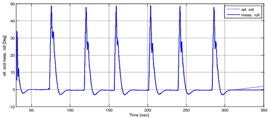
**Fig.19. Reference and measured Roll for 4 waypoints navigation**
