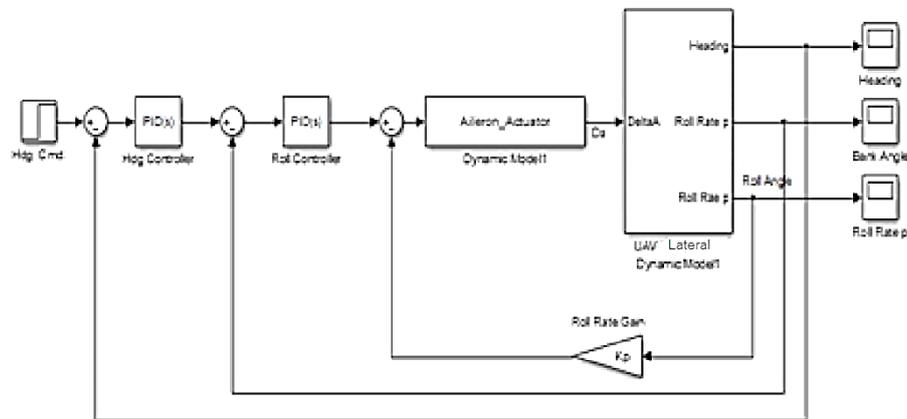
**Fig.8. Heading Controller**
