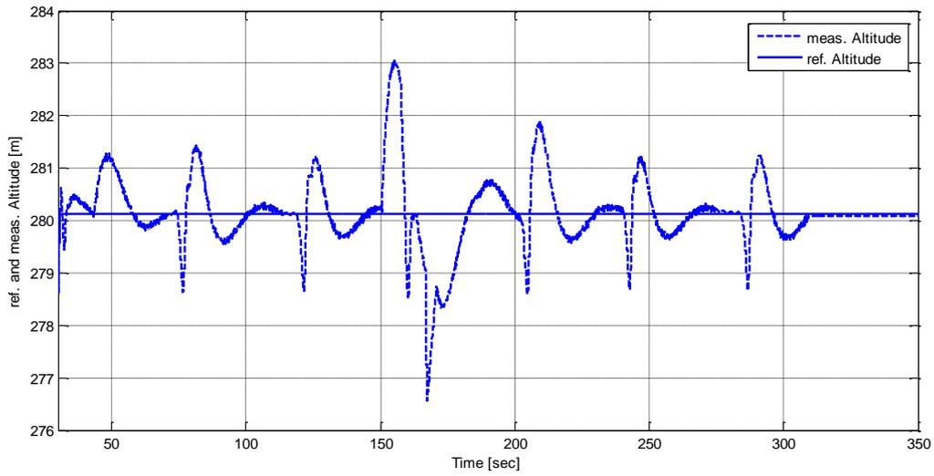
**Fig.17. Reference and measured Altitude for 4 waypoints navigation**
