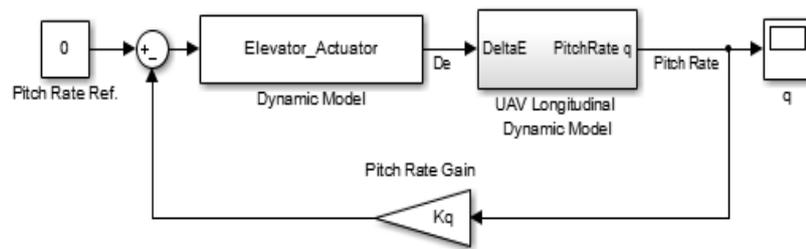
**Fig.10. Pitch Rate Controller**
