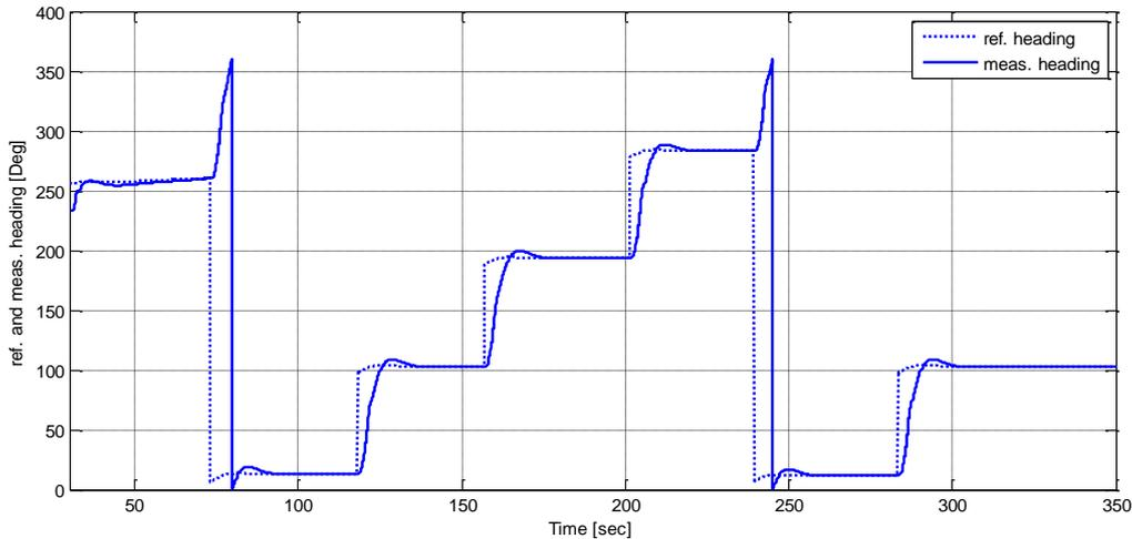
**Fig.20. Reference and measured heading for 4-WPnavigation**
