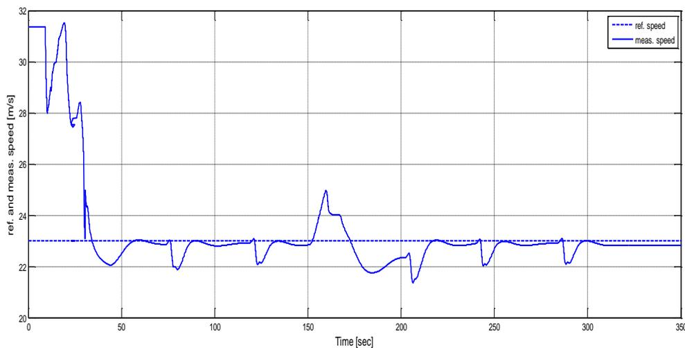
**Fig.21. Reference and measured Speed for 4 waypoints navigation**
