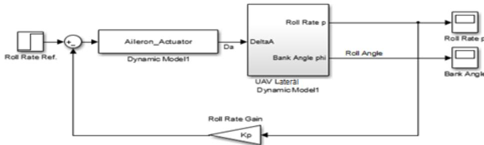
**Fig.6. Roll Rate Controller**
