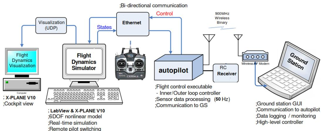
**Fig. 14. Hardware-In-Loop (HIL) Simulation Scheme**
