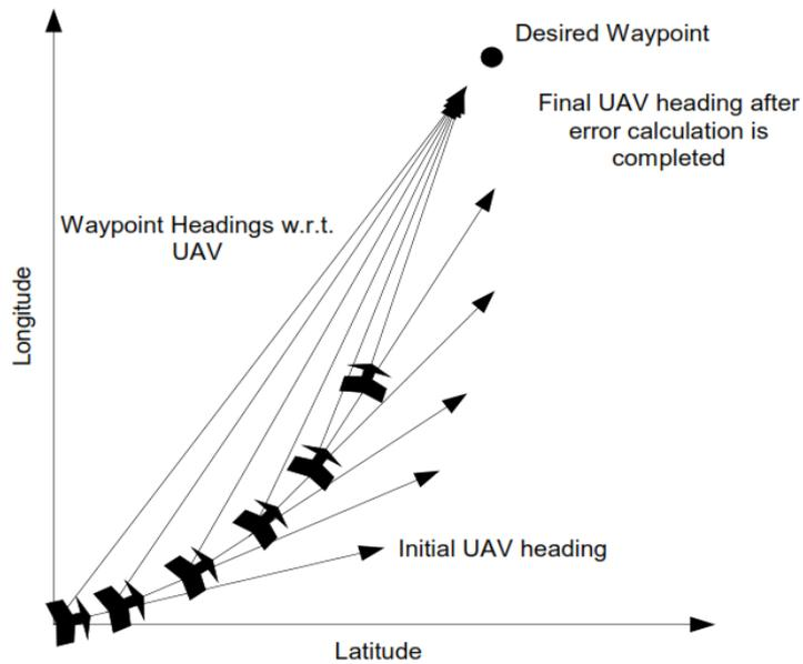
**Fig.2. Error Minimization Trajectory**
