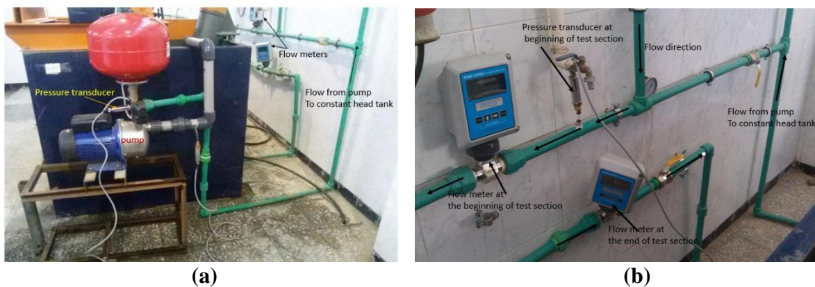
Fig. 7. (a) Test rig of the pipeline system, (b) Flowmeters and pressure transducer in fluid mechanics laboratory of the mechanical power and energy department.
