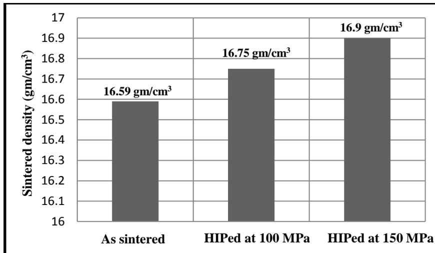
Fig.(14). Effect of HIPing pressure on the sintered density of the alloy 93% W-4.9%Ni-2.1%Fe, HIPed at 1300°C for 60minutes.
