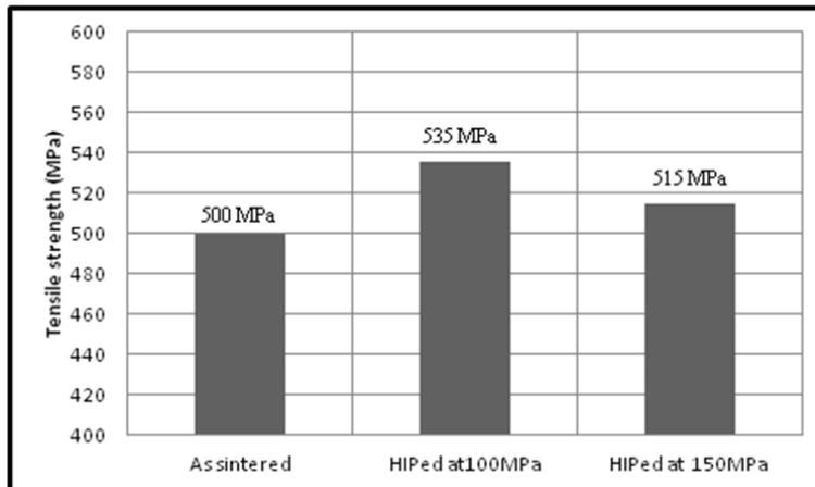
Fig.(9). Effect of HIPing pressure on the tensile strength of the alloy 93%W-4.9%Ni-2.1%Fe, HIPed at 1300°C for 60 minutes.
