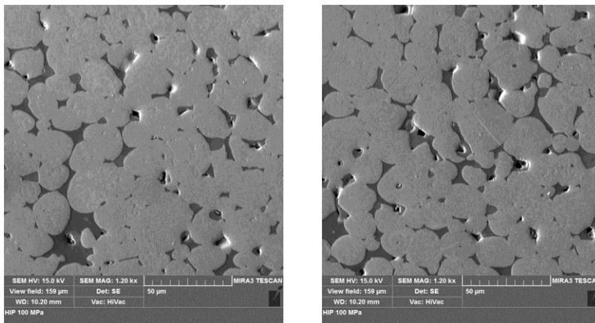
Fig.(6). SEM micrographs of the alloy 93%W-4.9%Ni-2.1%Fe CIPed at 200 MPa and sintered for 30 minutes at 1470°C, then HIPed at 1300°C under 100MPa for 60 minutes using magnification 1200X.
