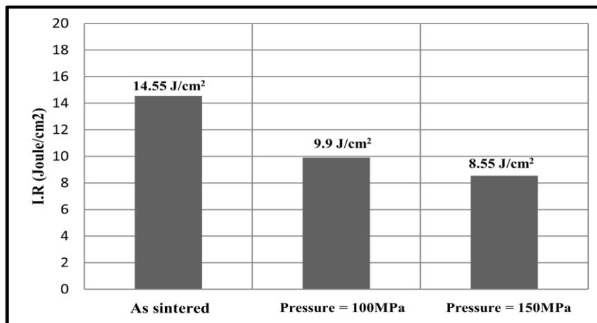
Fig.(11). Effect of HIPing pressure on the impact energy of the alloy 93%W-4.9%Ni-2.1%Fe, HIPed at 1300°C for 60 minutes.
