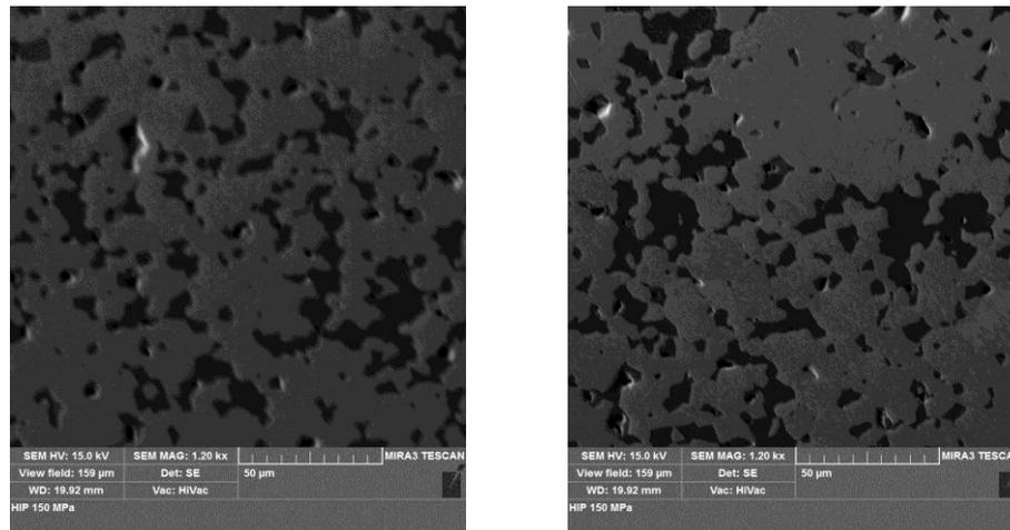
Fig.(7). SEM micrographs of the alloy 93%W-4.9%Ni-2.1%Fe CIPed at 200 MPa and sintered for 30 minutes at 1470°C, then HIPed at 1300°C under 150MPa for 60minutes using magnification 1200X.
