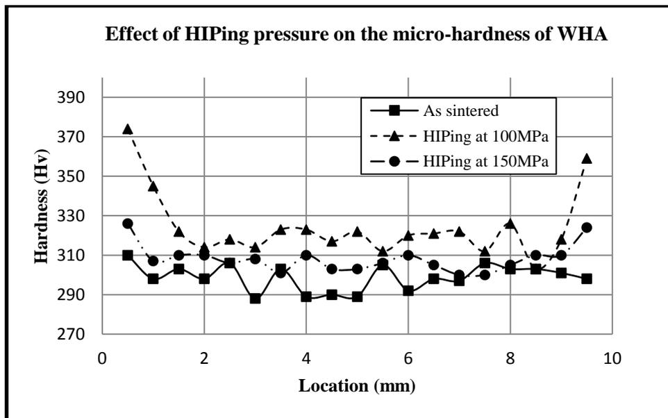
Fig.(13). Effect of HIPing pressure on the micro-hardness of the alloy 93%W-4.9%Ni-2.1%Fe, HIPed at 1300°C for 60minutes.
