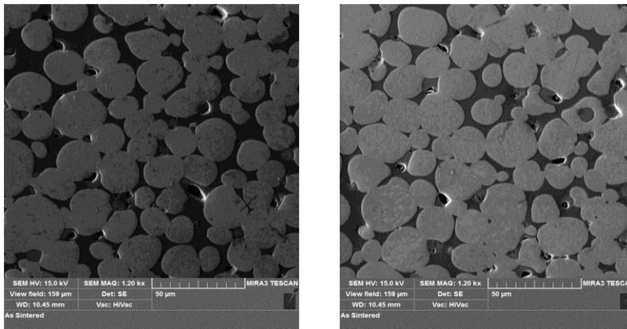
Fig.(5). SEM micrographs of the alloy 93%W-4.9%Ni-2.1%Fe CIPed at 200 MPa and sintered for 30 minute at 1470°C, using magnification 1200X.
