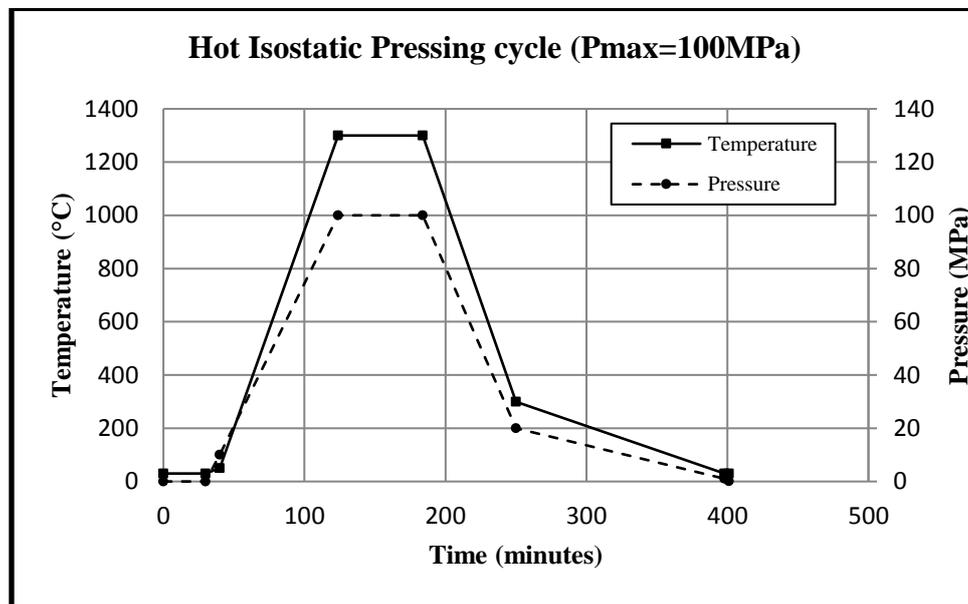
Fig.(2). HIP cycle applied for maximum pressure of 100 MPa.
