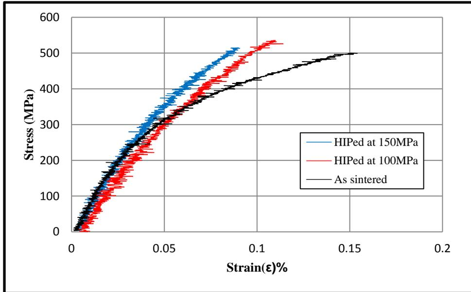
Fig.(8). Stress strain curves of the alloy 93%W-4.9%Ni-2.1%Fe in the as sintered state and after applying a HIPing cycle at 1300°C for 60minutes under an isostatic pressure of 100MPa and 150MPa.
