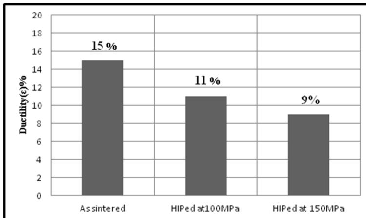
Fig.(10). Effect of HIPing pressure on the ductility of the alloy 93%W-4.9%Ni-2.1%Fe, HIPed at 1300°C for 60minutes.
