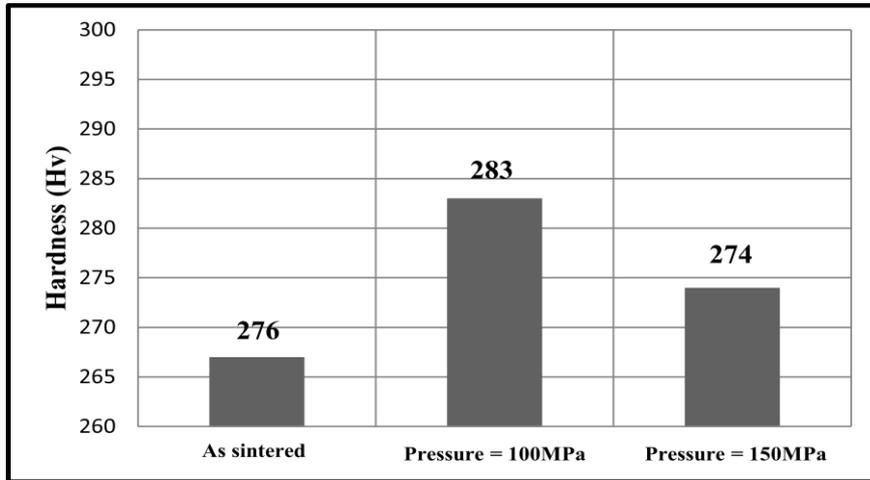
Fig.(12). Effect of HIPing pressure on the hardness of the alloy 93%W-4.9%Ni-2.1%Fe, HIPed at 1300°C for 60minutes.
