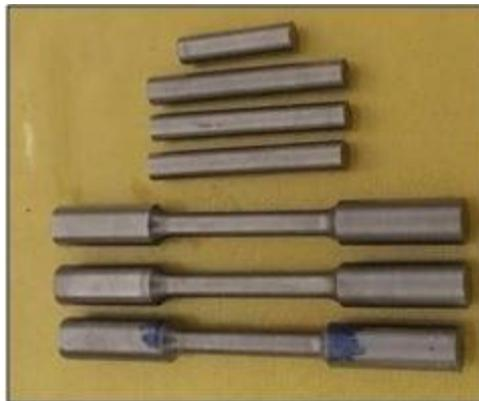
Fig.(4). The produced specimens used in determination of tensile strength, impact and sintered density after applying a HIPing cycle at 1300°C with different isostatic pressures.
