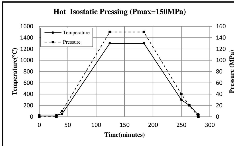
Fig.(3). HIP cycle applied for maximum pressure of 150 MPa .
