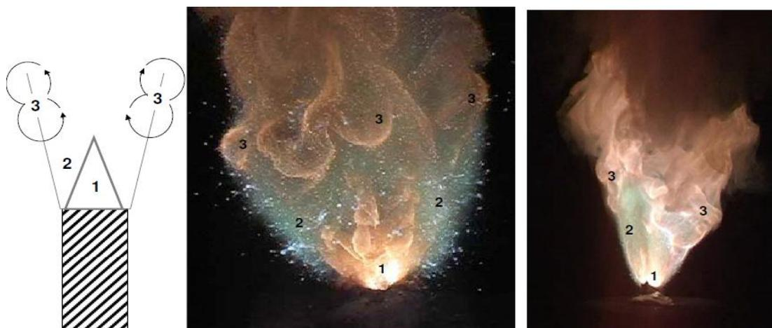
Fig. 8. Model for MTV flare combustion (a) with real photo-image for MTV flame (b, c)
