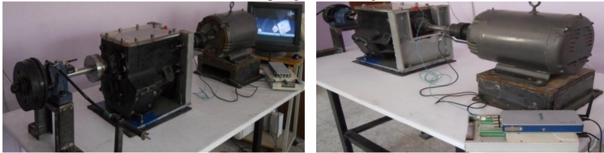
1. Inverter, 2. Electric motor, 3. Fixable coupling, 4. 130 mm centre distance Gearbox, 5. Mechanical coupling, 6. Loading Mechanism
