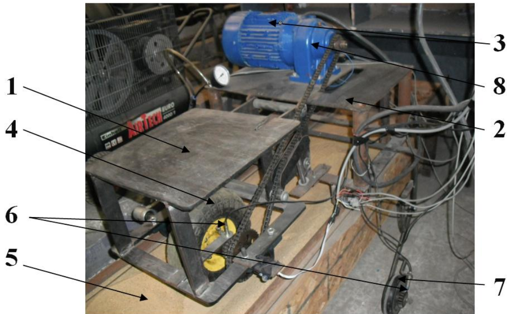
1-Moving carriage, 2-Towing trolley, 3-Electric motor, 4-Test tire, 5-Soil bin, 6-Speed sensor, 7-Ground wheel, 8-Gear Box
