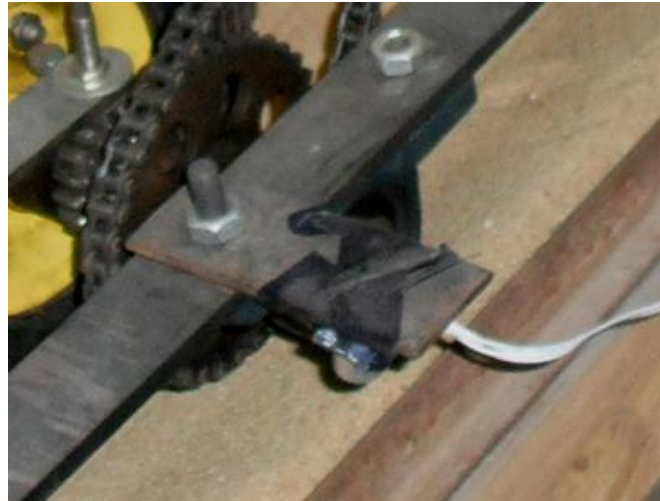
Fig. 5. Ultrasonic distance sensor
