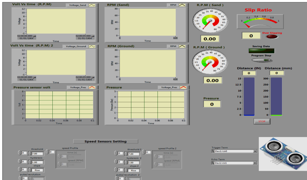
Fig. 15. Control panel Interface with LabView with all sensors
