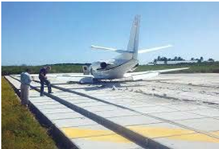
Figure 2. Tire-to-Foamcrete Interface Crushing, ultimately stopping aircraft
