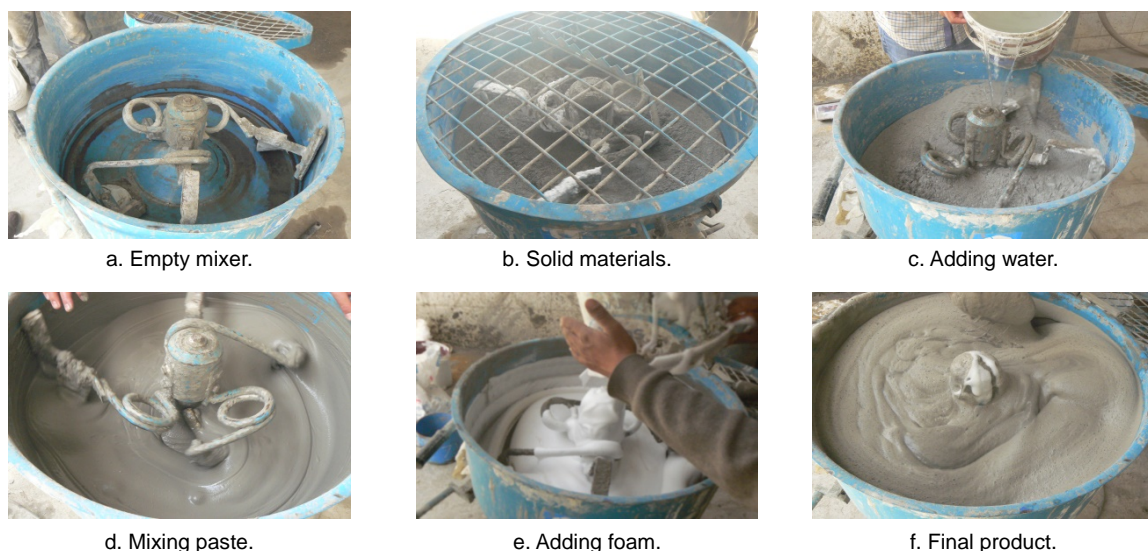
Figure 5. Foamed concrete manufacturing process.
