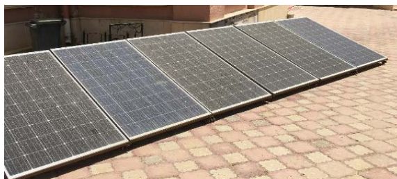
Figure 3: Tested solar panels held on 30° tilted holders facing South direction
