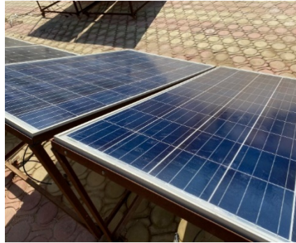
Figure 11: Solar Panel after applying the prepared Nano-coating
