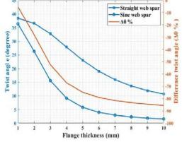
**Figure 17.**Twist angle due to torsion load on the straight-web and the sine-web for variable flange thickness.
