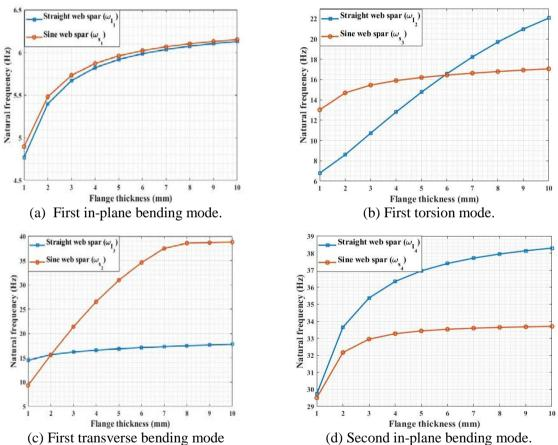
**Figure 19.** Mode shapes of straight and sine-web spars for variable flange thickness (straightweb thickness is 1mm and the sine-web thickness is 0.63542mm)
