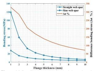
Figure 16. Bending stress on the straight-web and the sine-web for variable flange thickness.
