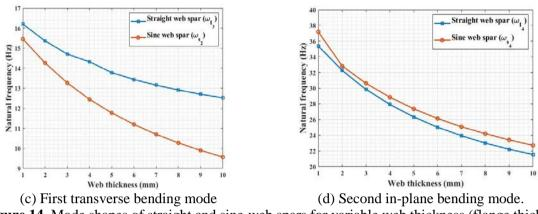
Figure 14. Mode shapes of straight and sine-web spars for variable web thickness (flange thickness is 3mm)
