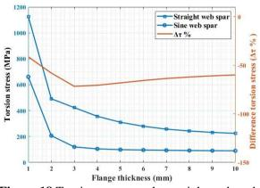
Figure 18. Torsion stress on the straight-web and the sine-web for variable flange thickness.
