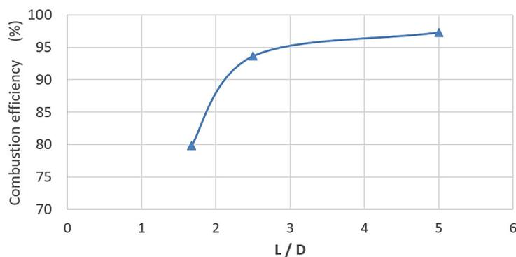
**Figure 22.** Influence of (L/D) ratio on combustion efficiency at GLR= 1 %, and  $p_{inj} = 1.5$  bar.
