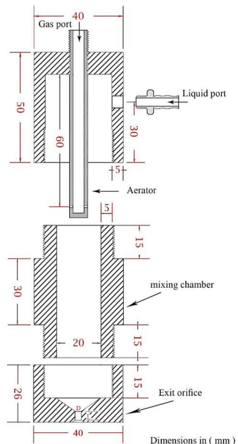
**Figure 1.** Schematic diagram of the tested effervescent atomizer.
