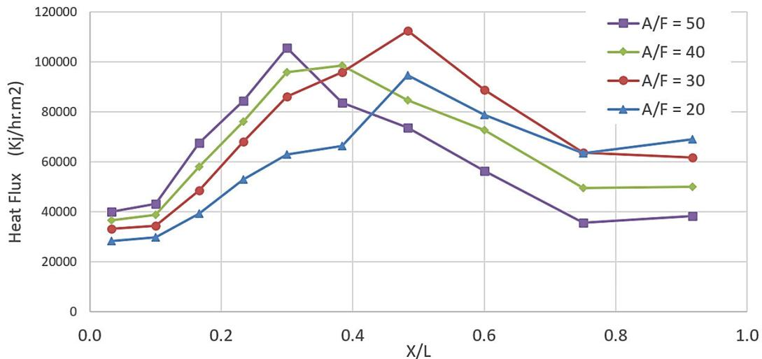
**Figure 5.** Total heat flux to the water jacket for different air to fuel ratio at GLR= 1 %, L/D= 2.5, and  $p_{inj} = 1$  bar.
