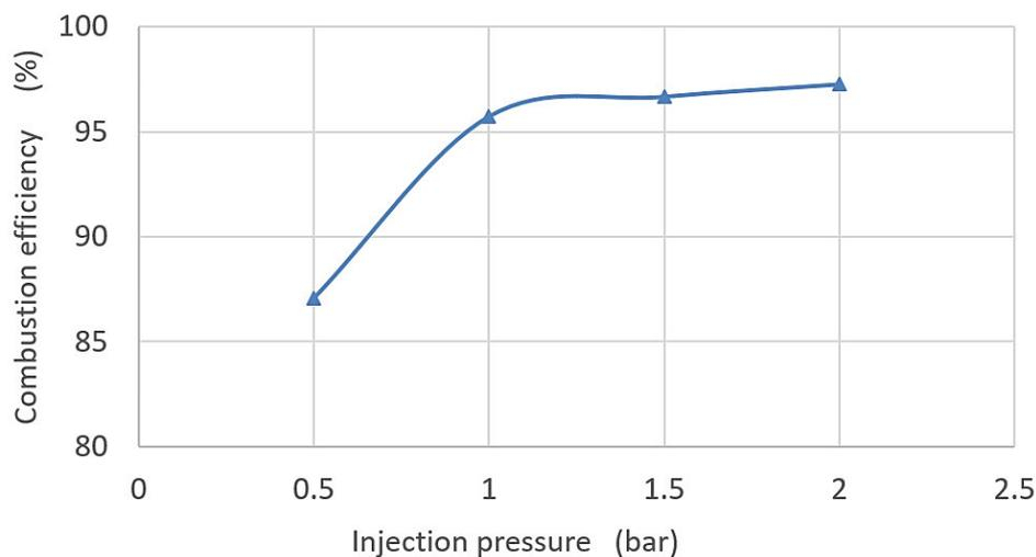
**Figure 17.** Influence of injection pressure on combustion efficiency at GLR = 1 %, L/D= 2.5, A/F= 40  $\text{Kg}_{\text{air}}/\text{Kg}_{\text{fuel}}$ .
