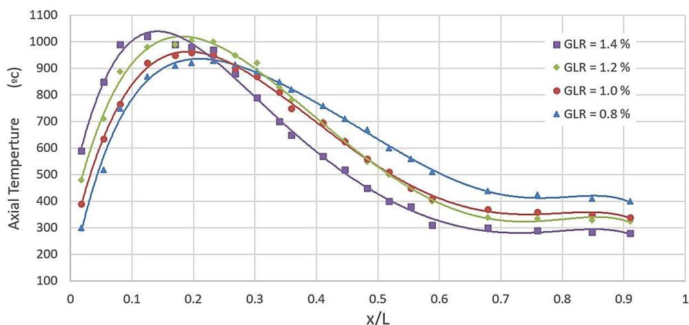
**Figure 8.** Influence of gas to liquid ratio on flame temperature distribution along the axis at A/F= 30 Kgair/Kgfuel,  $p_{inj} = 1.5$  bar, and L/D = 2.5
