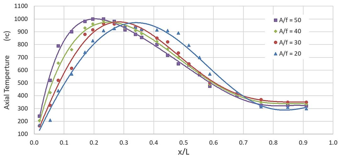
**Figure 3** Influence of air to fuel ratio on flame temperature distribution along the axis at  $p_{inj} = 1 \text{ bar}$ ,  $GLR = 1 \%$ , and  $L/D = 2.5$
