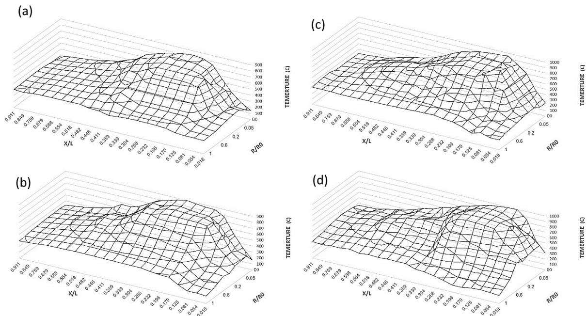
**Figure 14.** 3-D surface of flame temperature (°C) in the combustor at GLR= 1 %, L/D= 2.5, and A/F= 40 Kg<sub>air</sub>/Kg<sub>fuel</sub> a)  $p_{inj} = 0.5$  bar b)  $p_{inj} = 1$  bar c)  $p_{inj} = 1.5$  bar d)  $p_{inj} = 2$  bar.
