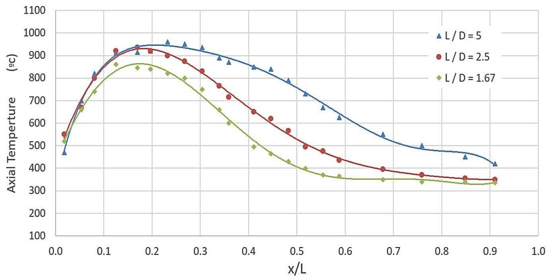
**Figure 18.** Influence of ( $L/D$ ) ratio on flame temperature distribution along the axis at  $A/F = 40 \text{ Kg}_{\text{air}}/\text{Kg}_{\text{fuel}}$ ,  $GLR = 1 \%$ , and  $p_{inj} = 1.5 \text{ bar}$ .
