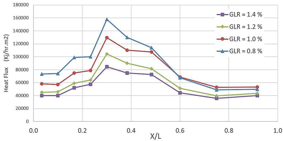
**Figure 10.** Total heat flux to the water jacket for different gas to liquid ratios at  $p_{inj} = 1.5$  bar,  $L/D = 2.5$ ,  $A/F = 30 \text{ Kg}_{air}/\text{Kg}_{fuel}$ .
