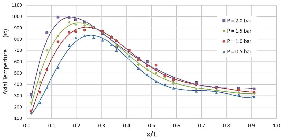
**Figure 13.** Influence of injection pressure on flame temperature distribution along the axis at  $A/F= 40 \text{ Kg}_{air}/\text{Kg}_{fuel}$ ,  $GLR= 1 \%$ , and  $L/D = 2.5$
