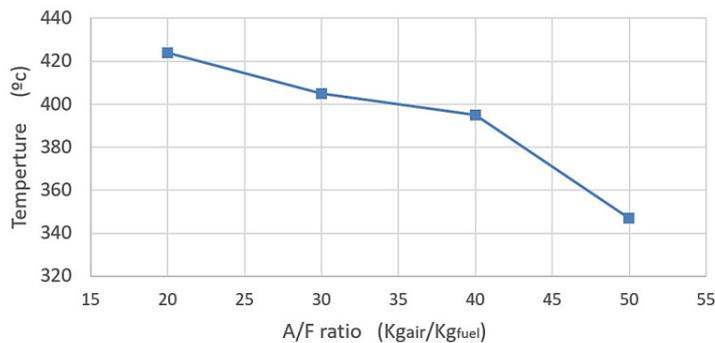
**Figure 6.** Stack temperature for different air to fuel ratio at GLR= 1 %, L/D= 2.5, and  $p_{inj} = 1$  bar.
