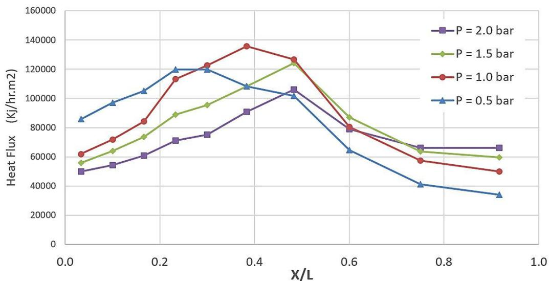
**Figure 15.** Total heat flux to the water jacket for different injection pressure at GLR = 1 %, L/D= 2.5, A/F= 40 Kg<sub>air</sub>/Kg<sub>fuel</sub>.
