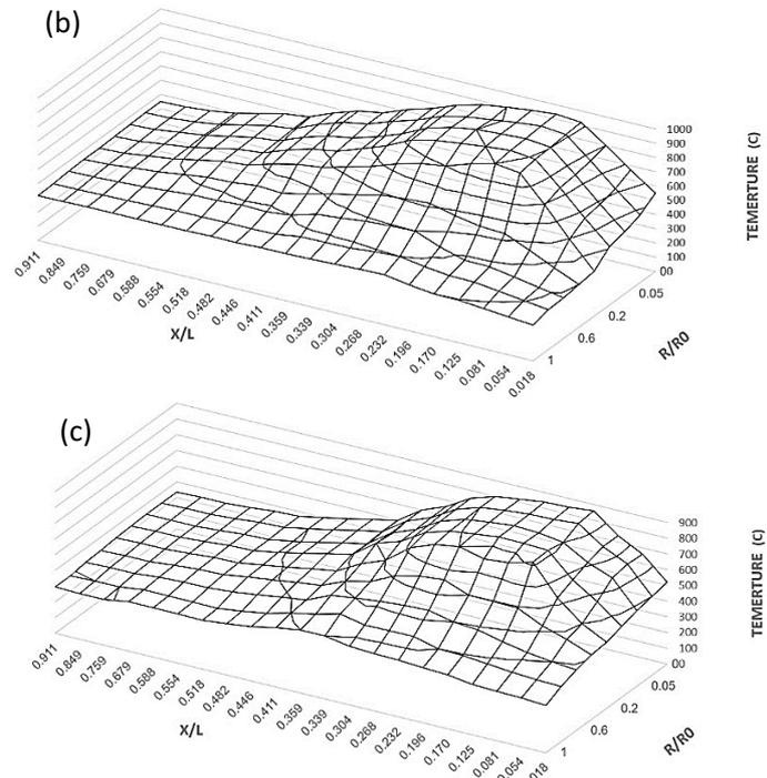
**Figure 19.** 3-D surface of flame temperature ( $^{\circ}\text{C}$ ) in the combustor at  $GLR = 1\%$ ,  $A/F = 40 \text{ Kg}_{\text{air}}/\text{Kg}_{\text{fuel}}$ , and  $p_{inj} = 1.5 \text{ bar}$  a)  $L/D = 5$  b)  $L/D = 2.5$  c)  $L/D = 1.67$
