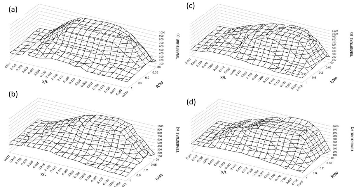
**Figure 4.** 3-D surface of flame temperature (°C) in the combustor at GLR= 1 %, L/D= 2.5, and  $p_{inj} = 1$  bar a) A/F= 20 b) A/F=30 c) A/F=40 d) A/F=50.
