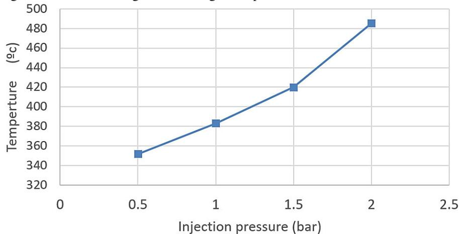
**Figure 16.** Stack temperature at different injection pressure at GLR= 1 %, L/D= 2.5, A/F= 40
