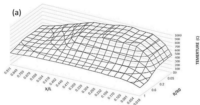
temperature at the flame zone and then a very low temperature at the other points outside the flame boundary. A uniform temperature region almost occurs in the outer recirculation zone and the temperature declines outside the flame boundary. Moving downward, the temperature profile becomes flat because of the measuring points lie outside the flame zone.
