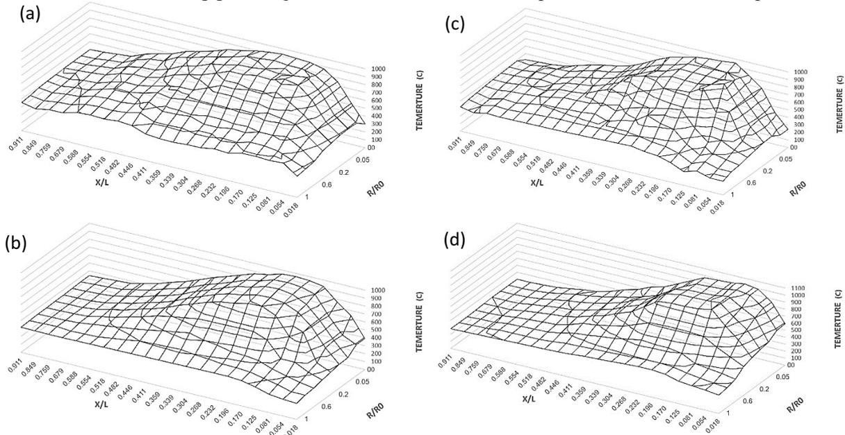
**Figure 9.** 3-D surface of flame temperature ( $^{\circ}\text{C}$ ) in the combustor at  $p_{inj} = 1.5 \text{ bar}$ ,  $L/D = 2.5$ , and  $A/F = 30 \text{ Kg}_{\text{air}}/\text{Kg}_{\text{fuel}}$  a)  $\text{GLR} = 0.8\%$  b)  $\text{GLR} = 1\%$  c)  $\text{GLR} = 1.2\%$  d)  $\text{GLR} = 1.4\%$ .
