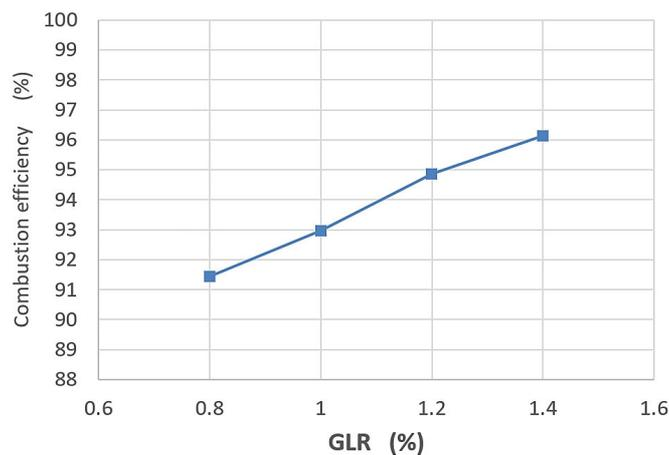
**Figure 12.** Combustion efficiency at different gas to liquid ratio at  $p_{inj} = 1.5$  bar,  $L/D = 2.5$ ,  $A/F = 30 \text{ Kg}_{air}/\text{Kg}_{fuel}$ .
