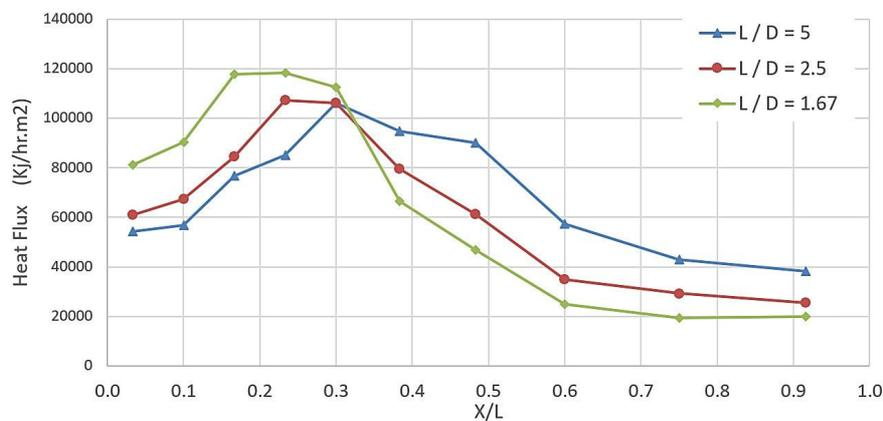
**Figure 20.** Total heat flux to the water jacket for different  $(L/D)$  ratio at  $GLR = 1\%$ ,  $A/F = 40 \text{ Kg}_{\text{air}}/\text{Kg}_{\text{fuel}}$ , and  $p_{inj} = 1.5 \text{ bar}$ .
