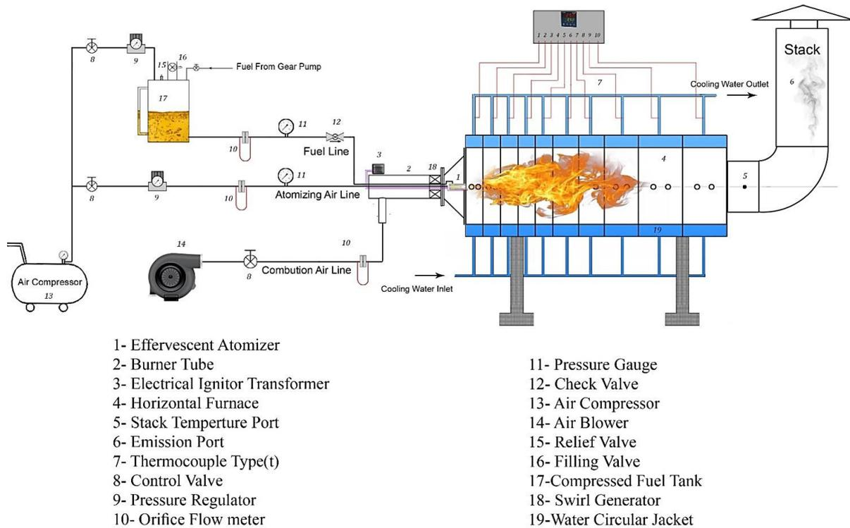
**Figure 2.** schematic diagram of the experimental test rig
