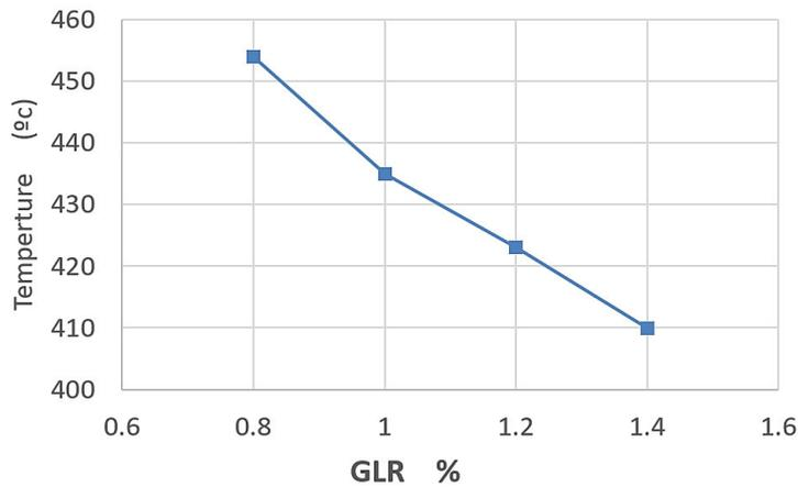
**Figure 11.** Stack temperature at different gas to liquid ratio at  $p_{inj} = 1.5$  bar,  $L/D = 2.5$ ,  $A/F = 30 \text{ Kg}_{air}/\text{Kg}_{fuel}$ .
