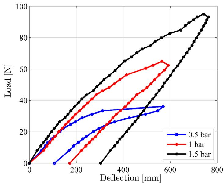
**Figure 4.** The load deflection curve of 20cm diameter beam
