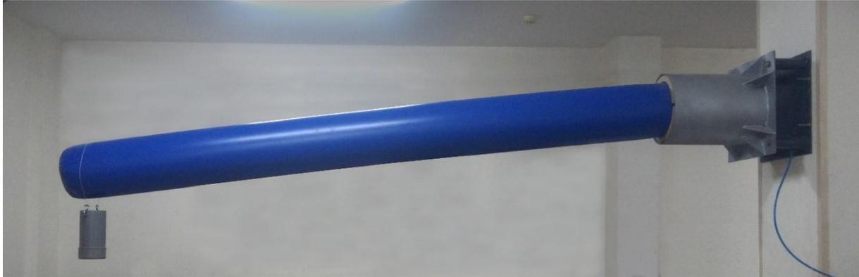
**Figure 3.** Inflatable beam under loading
