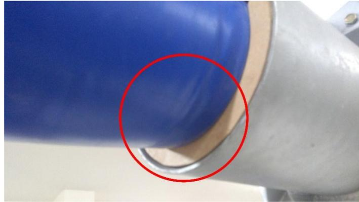
**Figure 7.** Beam wrinkling phenomenon
