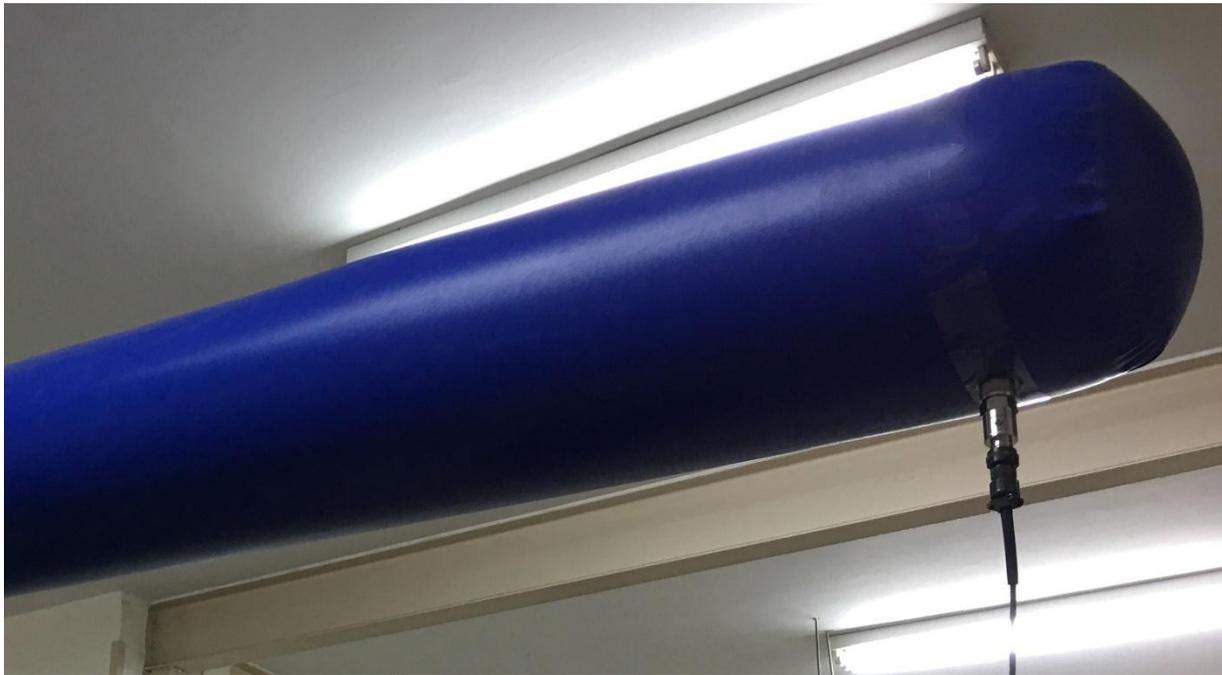
**Figure 8.** Device accelerometer attached to the inflatable beam
