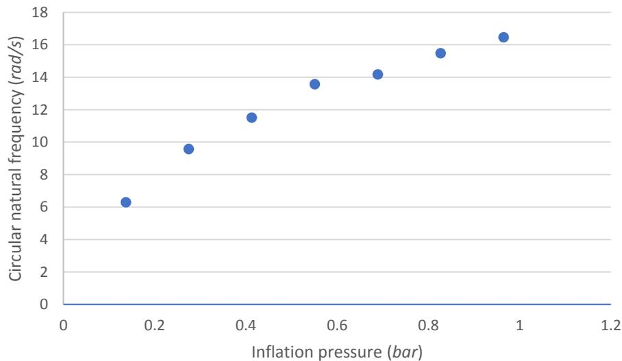
**Figure 10.** Circular natural frequency vs. inflation pressure
