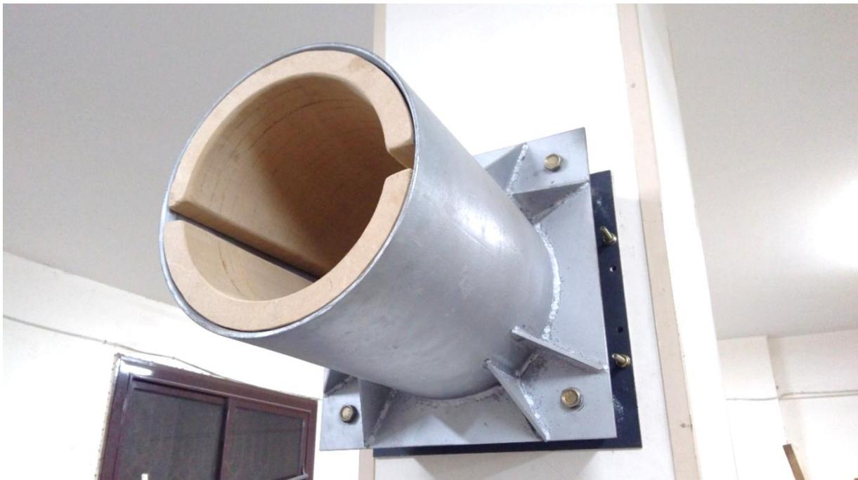
**Figure 2.** Inflatable beam test rig with beam adaptor.
