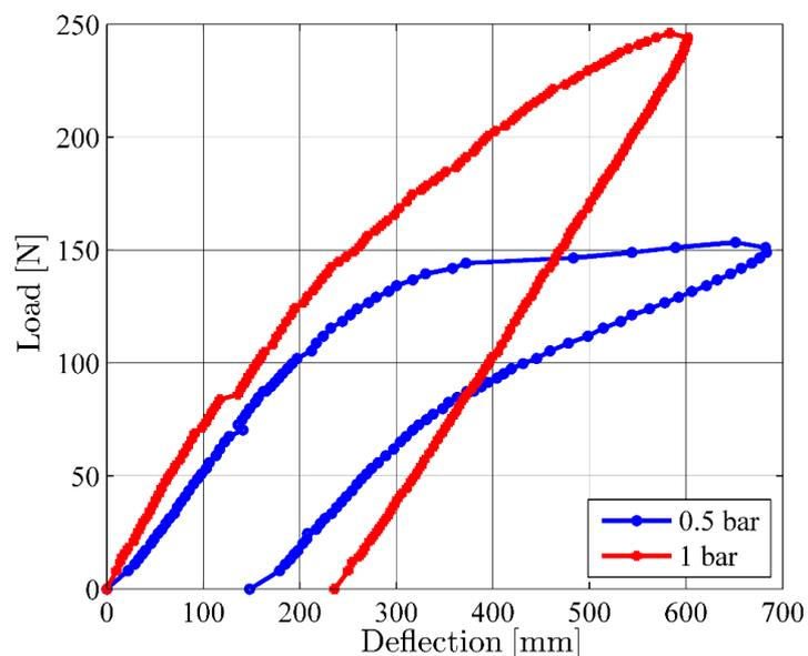
**Figure 6.** The load deflection curve of 30cm diameter beam
