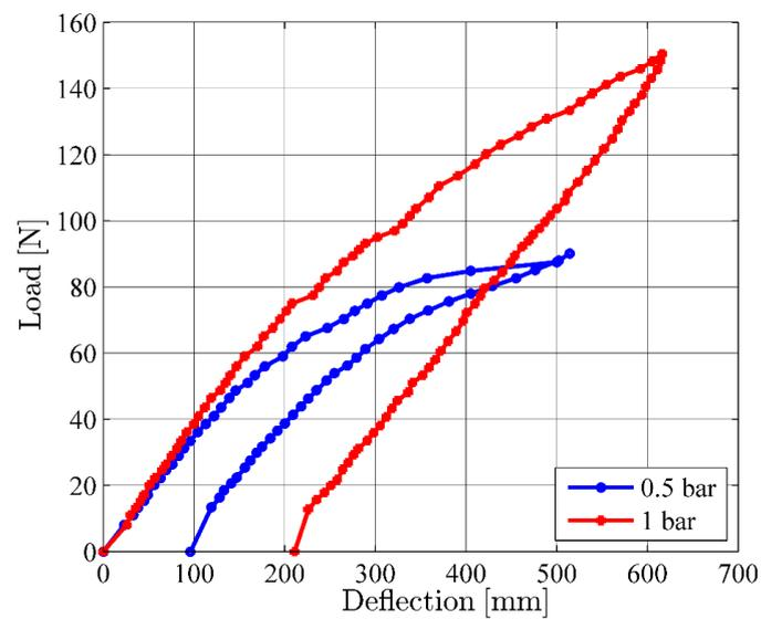
**Figure 5.** The load deflection curve of 25 cm diameter beam
