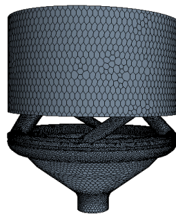
Figure 5. Mesh generation in the injector
