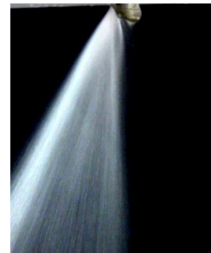
Figure 9: Side view of the fully developed spray
