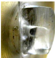
Figure 4: Acrylic sprayer showing the outlet hole of cut-angle 70^\circ
