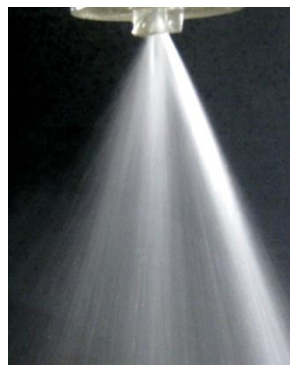
Figure 8: Frontal view of the fully developed spray
