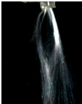
Figure 7: typical tulip shape of the spray at a low injection pressure
