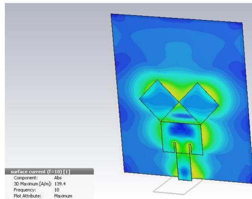
**Figure 16** surface current at frequency 10 GHz
