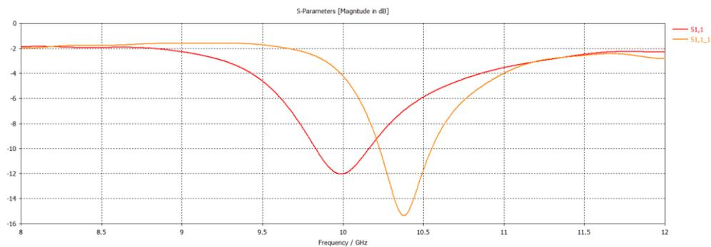
**Figure 8** return loss of first and second Pythagorean iterations, the red is iteration one and the orange is iteration two
