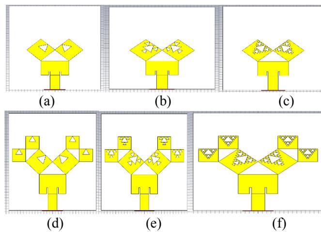
**Figure 5** shows the Sierpinski gasket iterations applied on the Pythagorean iterations
