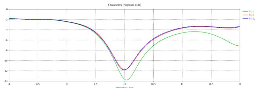
**Figure 9** return loss of first, second, third iteration Sierpinski on first iteration Pythagorean
