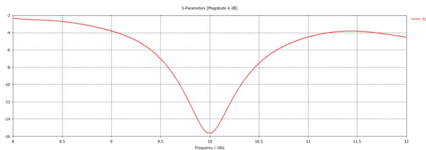
**Figure 11** return loss of conventional patch with Koch on sides
