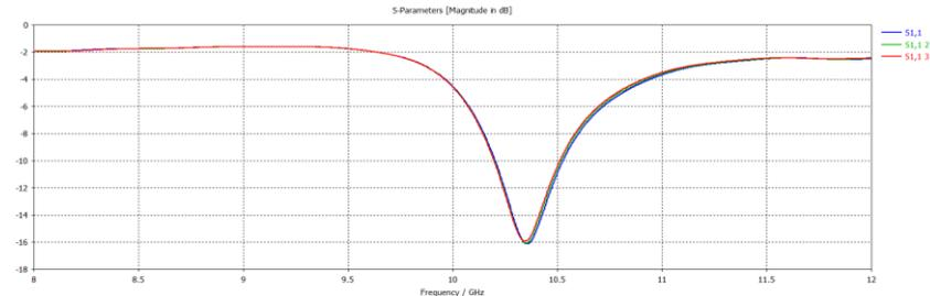
**Figure 10** return loss of first, second, third of Sierpinski applied on the second iteration Pythagorean
