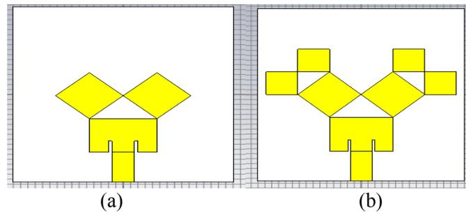
**Figure 4** Pythagorean first and second iteration applied on the conventional patch
