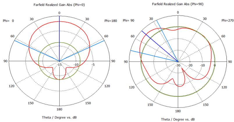
**Figure 14** 2D radiation pattern of first iteration Pythagorean at resonant frequency of 10 GHz
