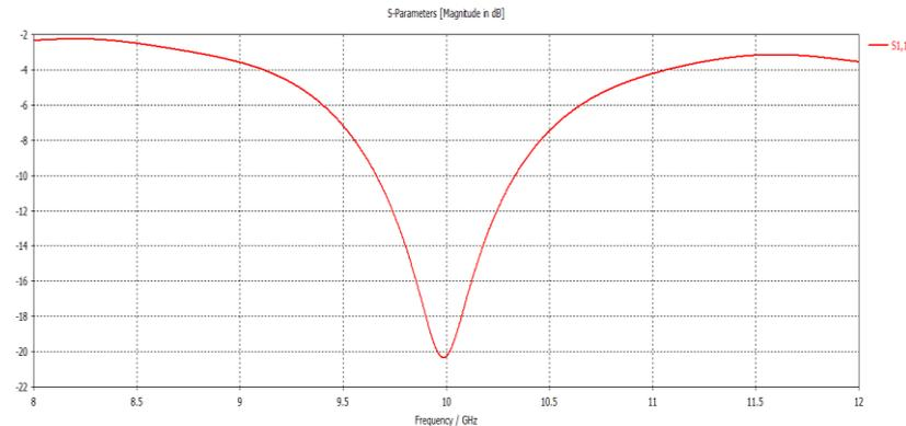
**Figure 7** Return loss of the conventional patch
