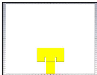
**Figure 3** Conventional patch antenna
