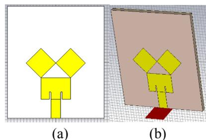
**Figure 12** Top and Perspective View of first iteration Pythagorean antenna designed on CST.
